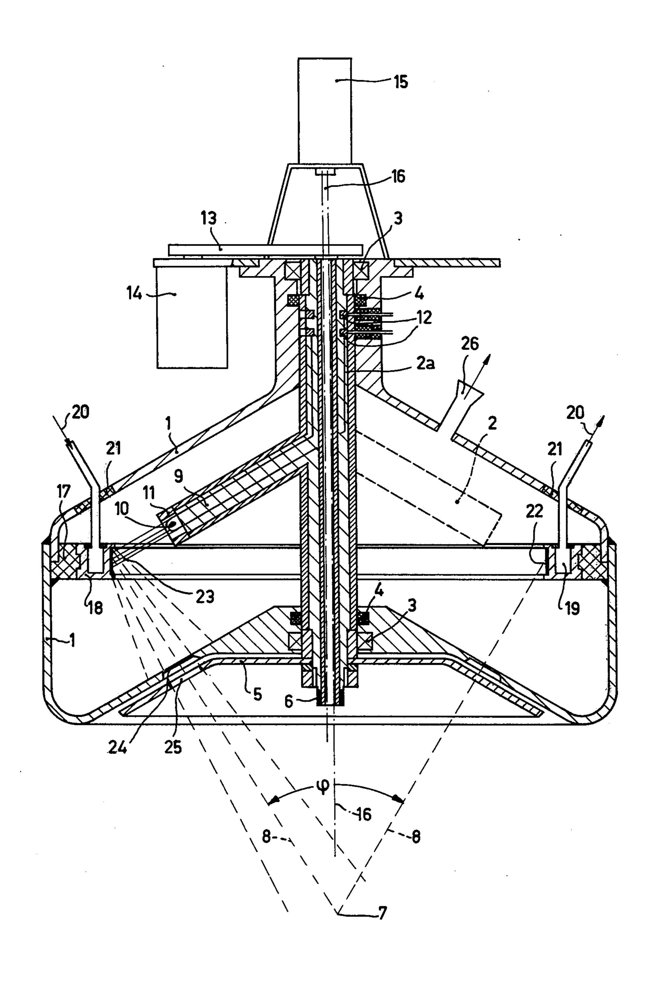
The invention relates to an X-ray source comprising drive means for realizing relative movement between a cathode and an anode of the source.
