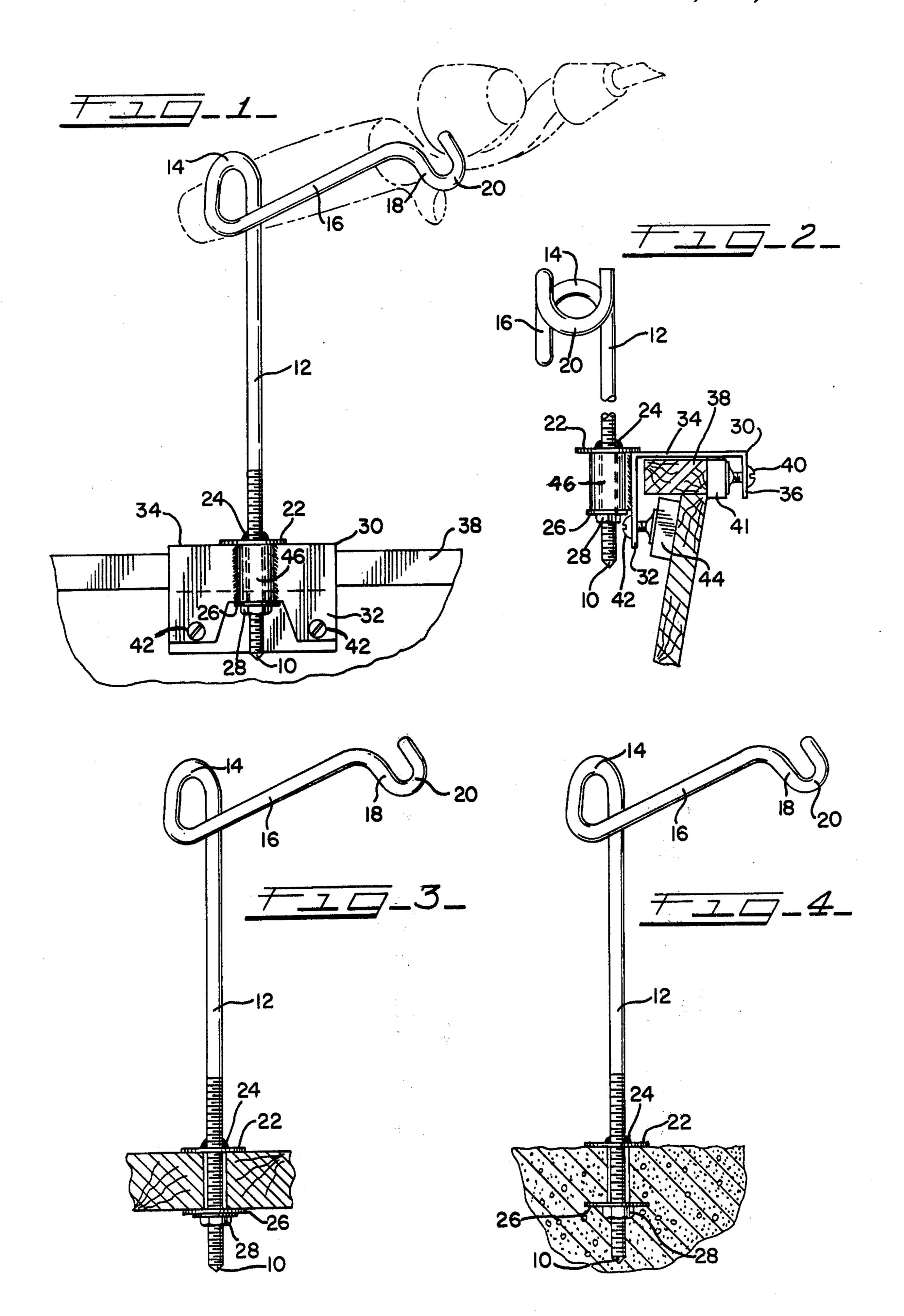
thereon by the lock nut 28, and press it into the sand, for further stability of the holder, as shown in FIG. 4.
