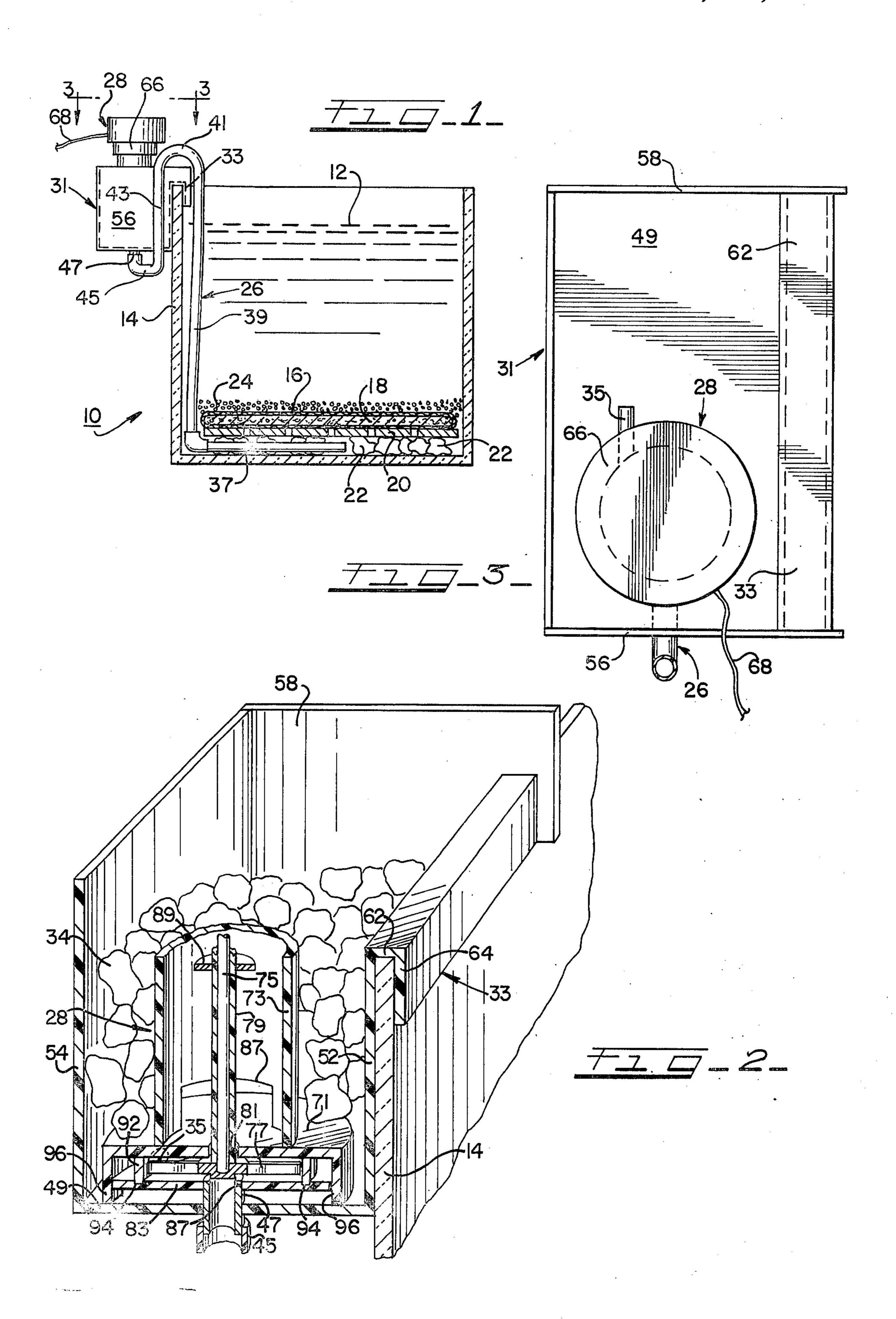
ably composed of non-metallic material, such as plastic, so that the wetted surfaces are not corrosive.
