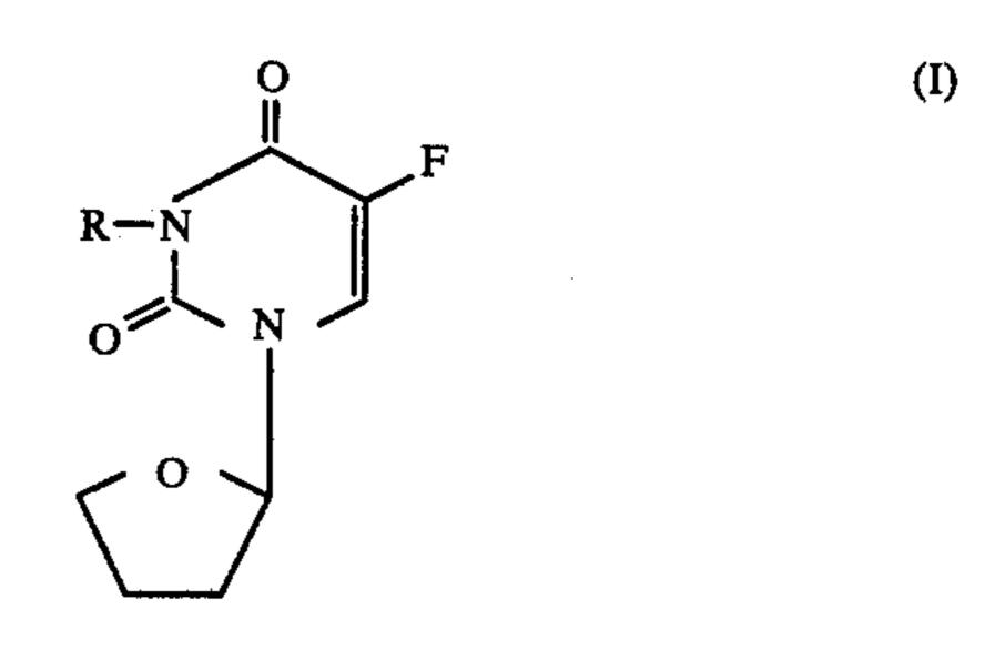
wherein R represents hydrogen atom or 2-tetrahydrofuryl group is produced by reacting more than equi-mole of 2,3-dihydrofuran with 5-fluorouracil in a polar aprotic solvent with a catalytically effective amount of a catalyst selected from the group consisting of metal halides, non-metal halides, tertiary amine salt of inorganic acids and organic acids in neutral or basic condition at 50° to 150° C under pressure.
