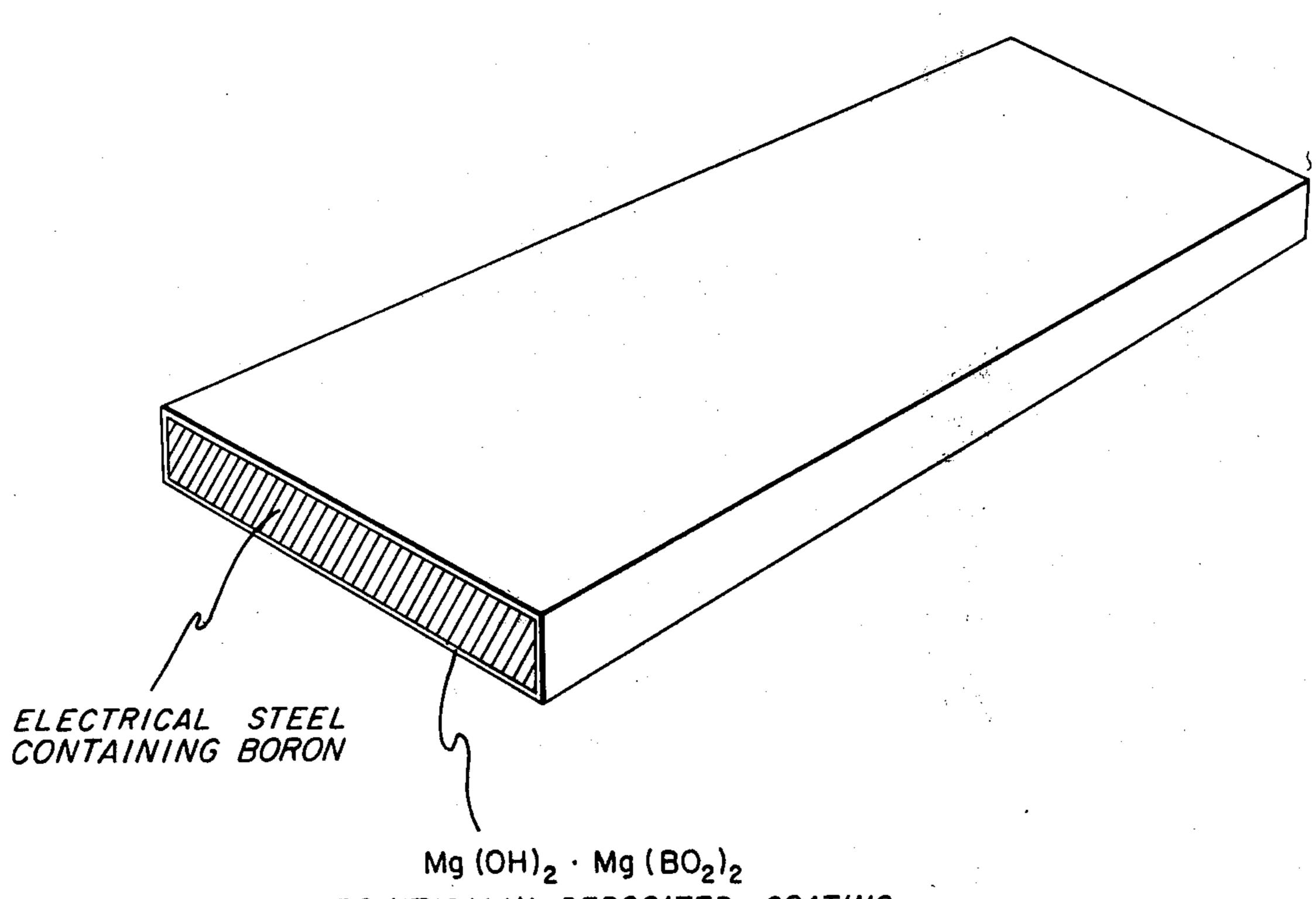
ELECTROLYTICALLY DEPOSITED COATING
