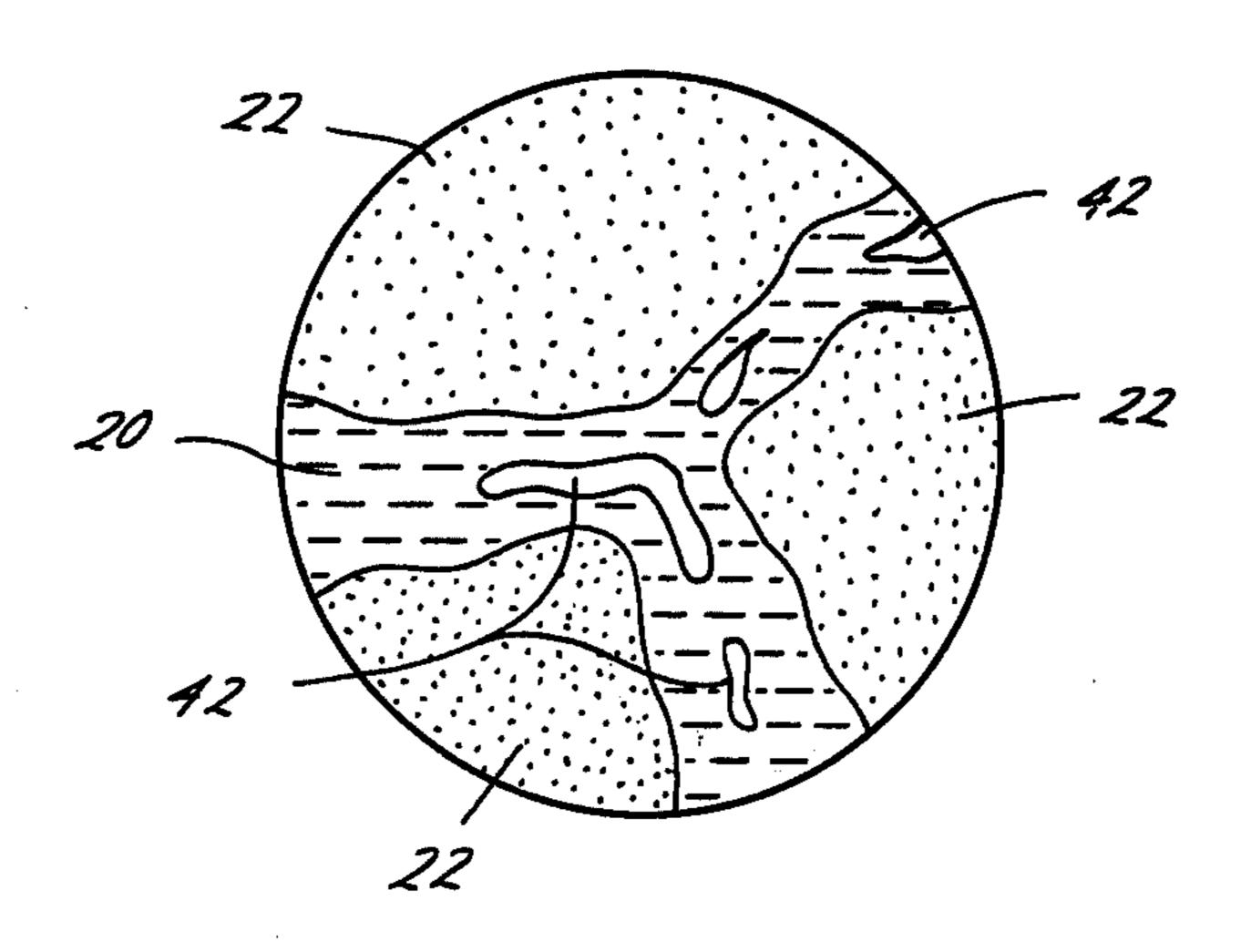
SAND, HAVING A CONTINUOUS FREE GAS PHASE WITHIN THE CONNECTED PORES BETWEEN WATER WETTED SAND GRAINS
