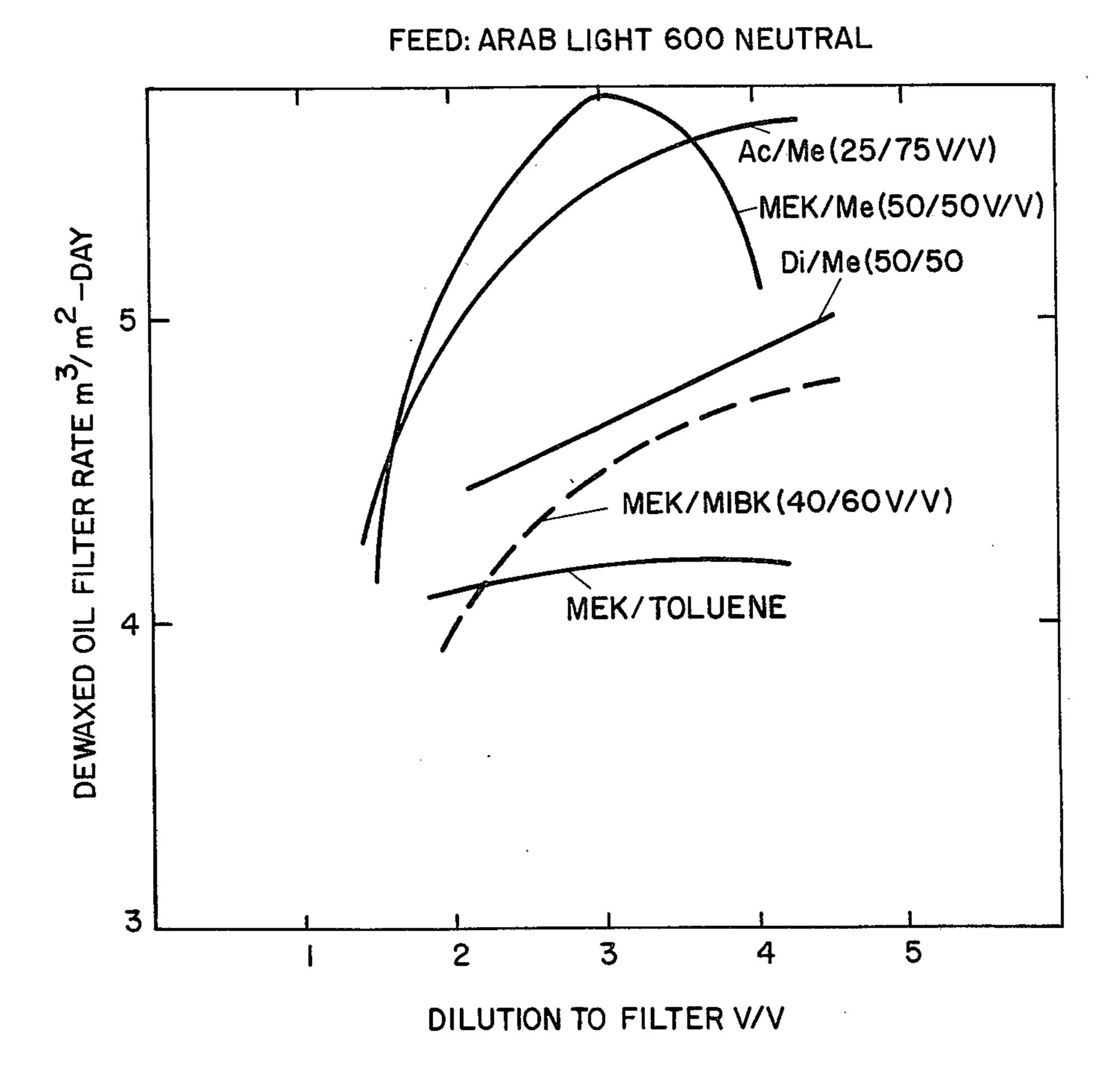
FIGURE 4 DEWAXED OIL FILTER RATE COMPARISON FOR MEK/MEAND MEK/MIBK DEWAXING SOLVENTS
