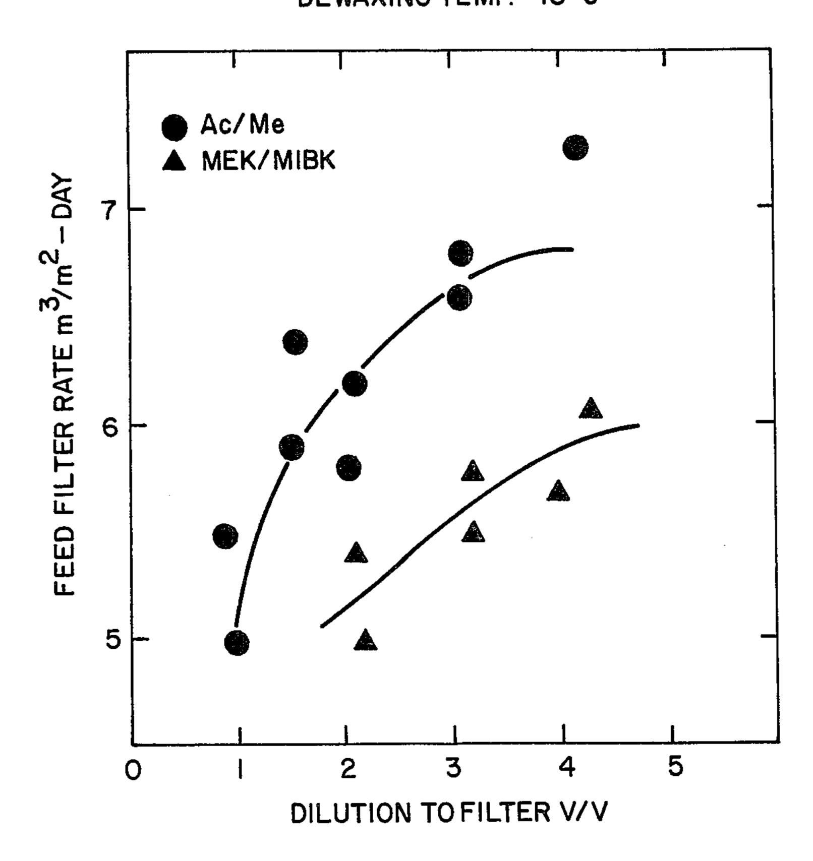
FIGURE 3 DEWAXED OIL FILTER RATE COMPARISON FOR Di/Me, Ac/Me, AND MEK/Me MEK/MIBK MEK/TOLUENE
