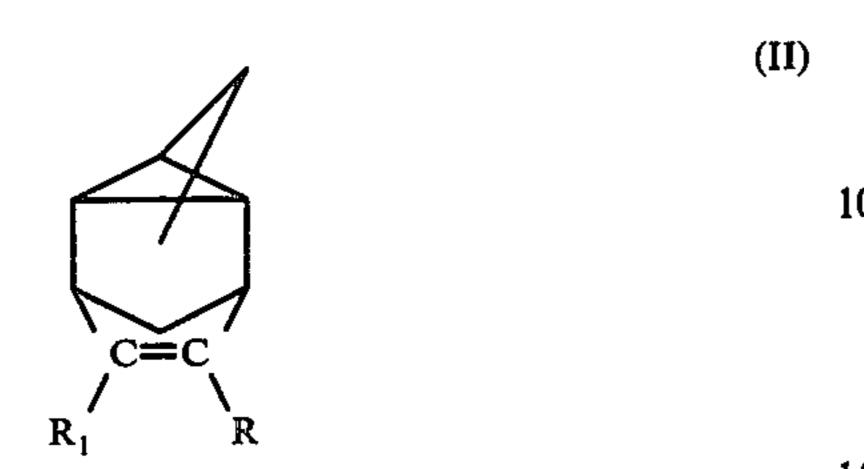
In structure II  $R_1$  and R are interchangeable. Examples of  $R_1C \equiv CR$  include propyne, butyne, pentyne-1, heptyne, octyne, decyne, pentyne-2, 3 methylbutyne-1, hexyne-2 and hexyne-3.
