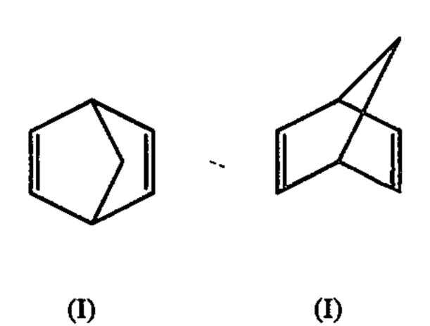
NBD can be easily dimerized to an hexacyclic dimer. Thus one problem in reacting NBD with another hydrocarbon reactant is to minimize the formation of the 50 foregoing dimer while encouraging the formation of the desired codimer.
