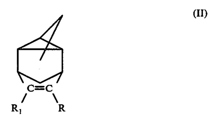
wherein  $R_1$  is a  $C_1$ - $C_{10}$  paraffinic or iso alkyl and R is a hydrogen or a  $C_1$ - $C_{10}$  paraffinic or iso alkyl and wherein R and  $R_1$  are interchangeable as to their location on the structure.
