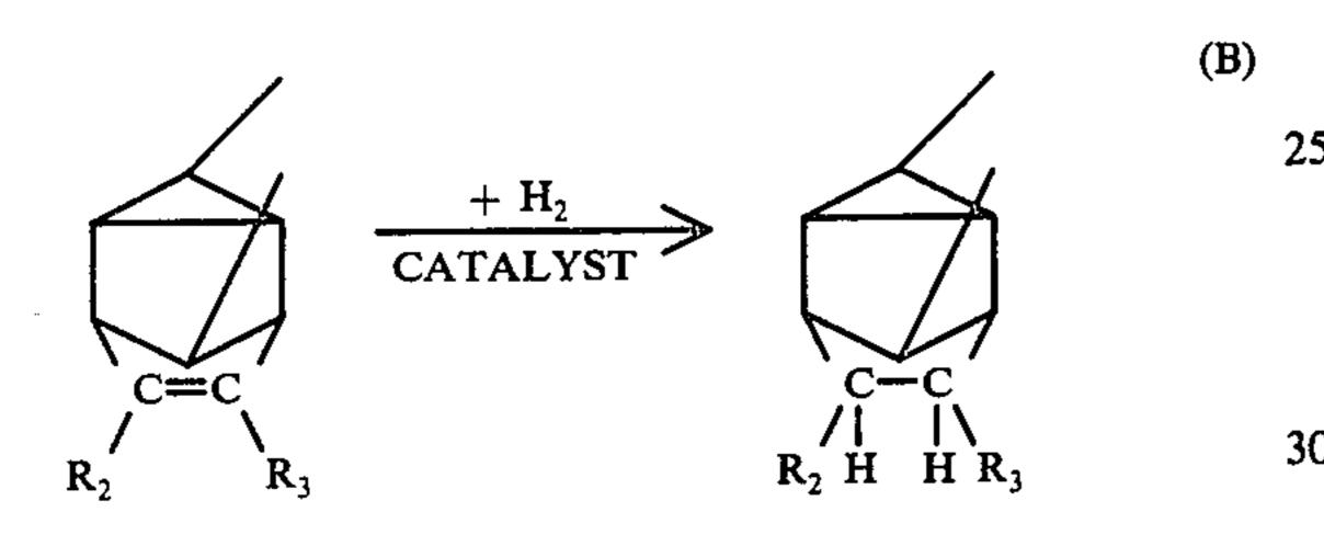
wherein each  $R_2$  and  $R_3$  are a  $C_1$ – $C_{10}$  paraffinic or iso alkyl or hydrogen. As an example the hydrogenation of the codimer deltacyclene (III) yields deltacyclane (IV). The latter two codimers have the following structure:
