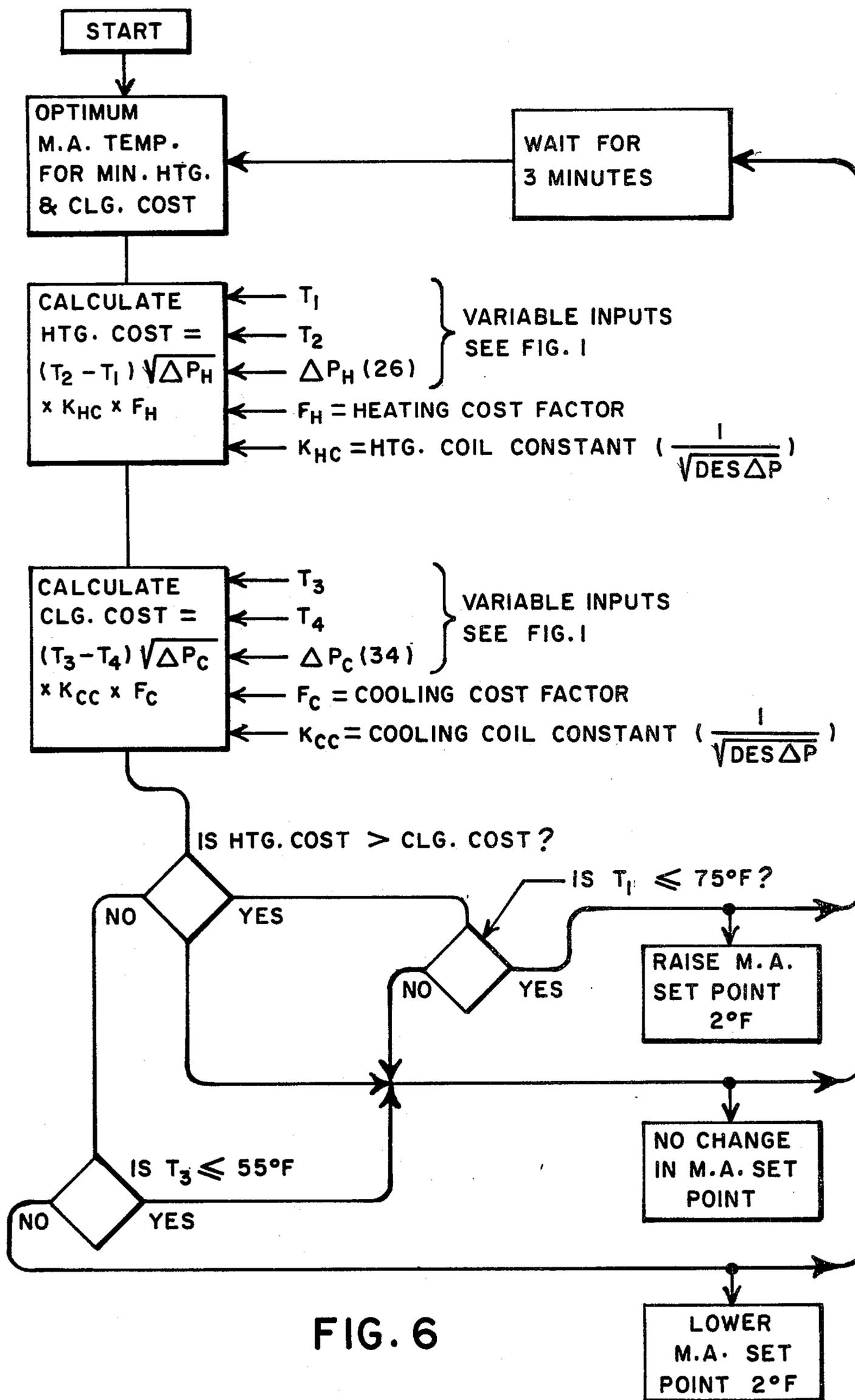
**HEATING AND COOLING COST MINIMIZATION****BACKGROUND OF THE INVENTION**
