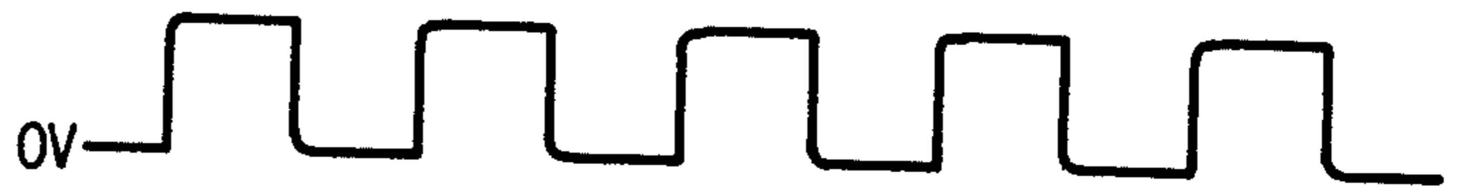
FIG. 3a ASTABLE MULTIVIBRATOR
