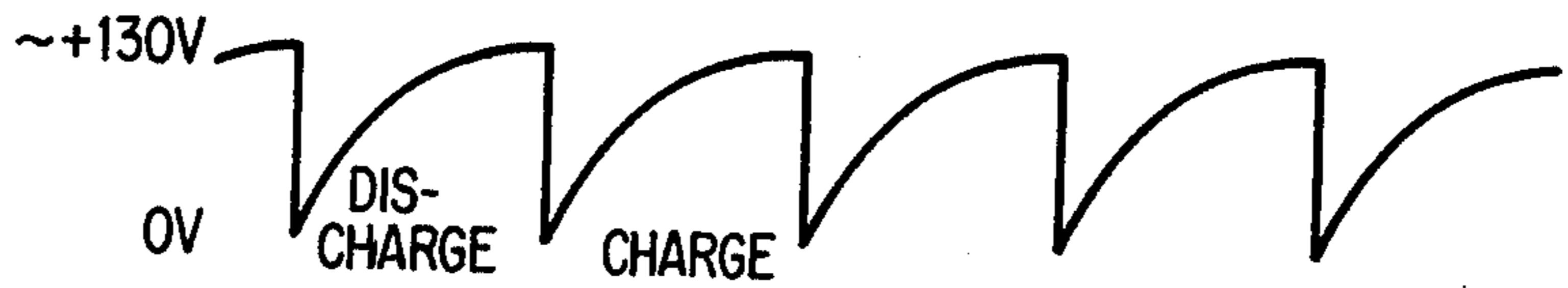
FIG. 3d CHARGE/DISCHARGE CYCLE OF H.V. PULSES TRANSMITTER
