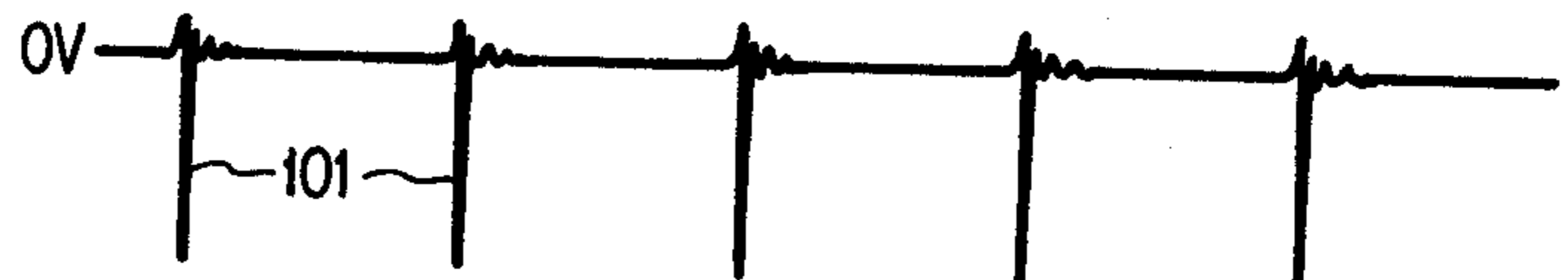
FIG. 3e H.V. PULSE TRANSMITTER OUTPUT TO TRANSDUCER
