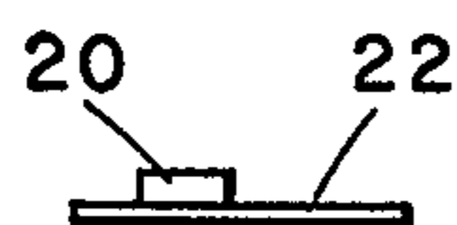
MOUNT LED ON APERTURED CONDUCTIVE TAPE.
