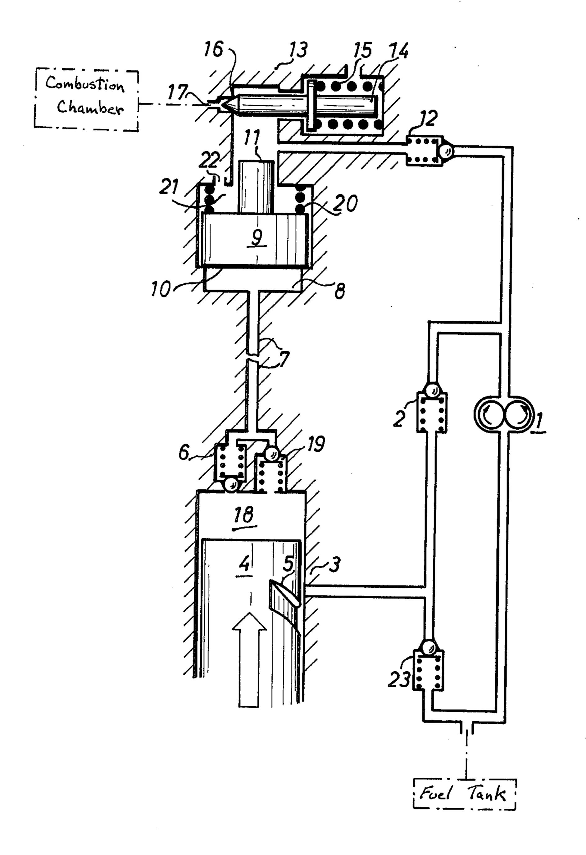
16 in the closed position by a valve spring 15. The injection opening 17 leads to the combustion chamber.
