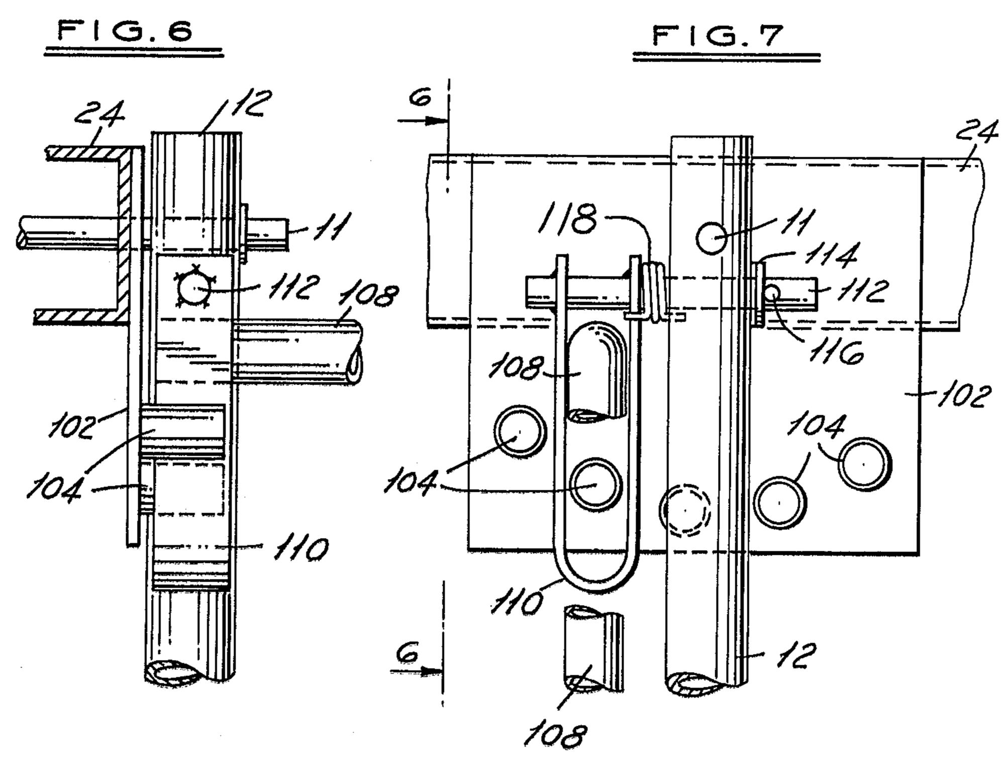
FIGS. 6 and 7 are respective front and side views of means for adjusting the elevational angle of the apparatus illustrated in FIGS. 1-3, FIG. 6 being a sectional view taken along the line 6—6 in FIG. 7.
