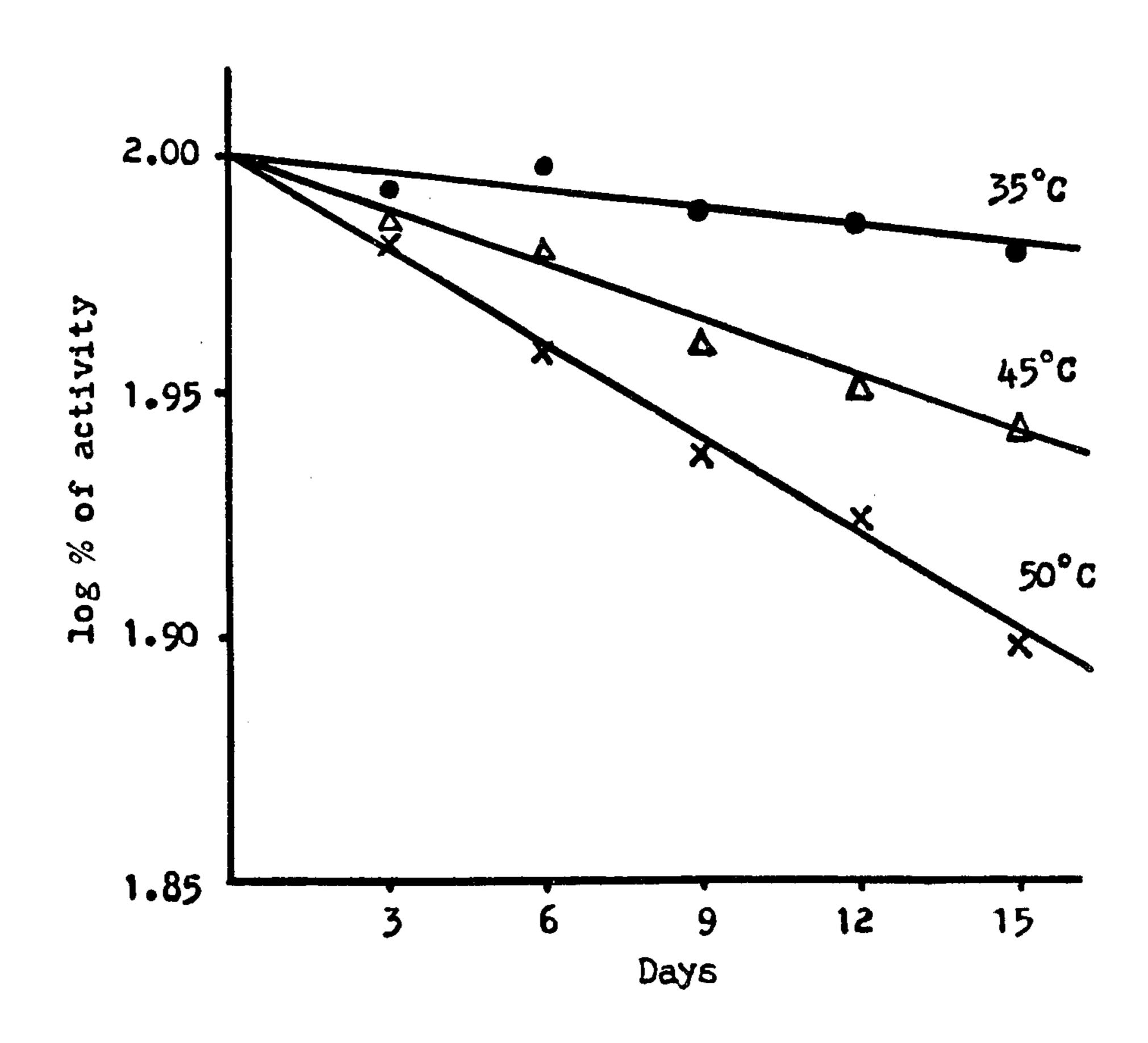
FIG. 2 Arrhenius Plots of MCR Lyophilized with Maltose
