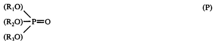
wherein  $R_1$ ,  $R_2$  and  $R_3$  are each a hydrocarbon radical having from 6 to 8 carbon atoms. Accordingly,  $R_1$ ,  $R_2$  and  $R_3$  each can be an octyl, 2-ethylhexyl, 2,2,4-trimeth-
