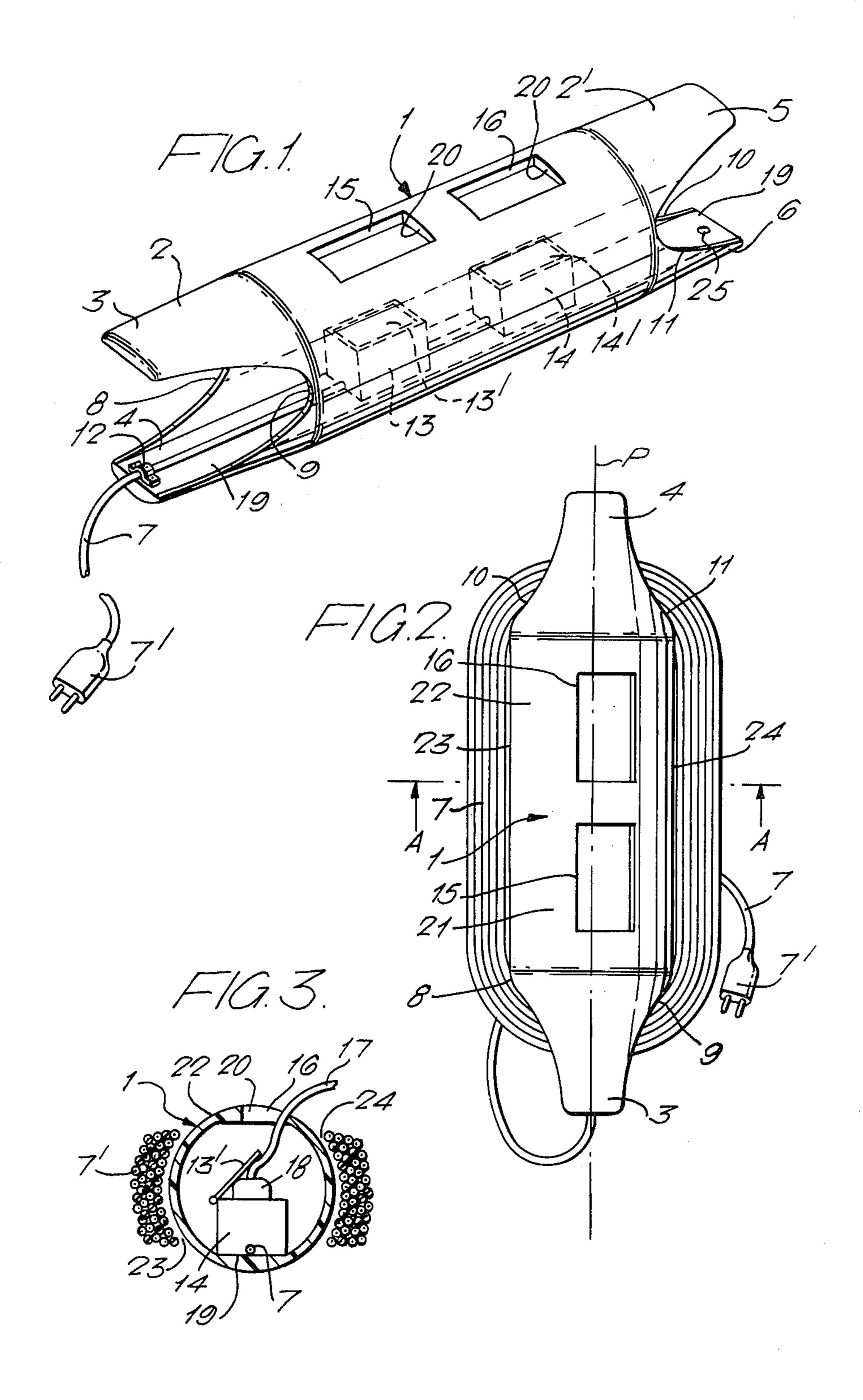
two oppositely directed flaps and also serve as access openings to the equipment in the interior of the housing.
