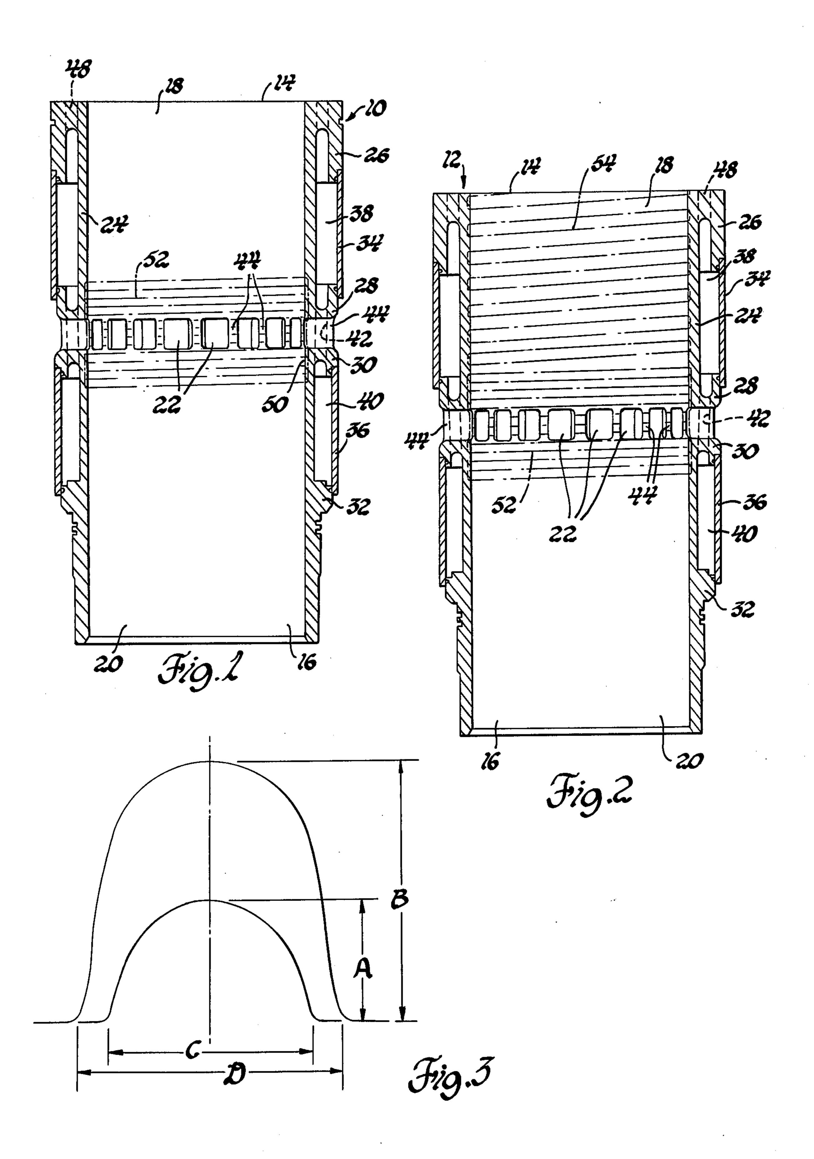
ening to provide selective case hardening of the port relief areas and, optionally, the upper cylinder bores of ported engine cylinders, particularly of the type represented by cast water jacketed cylinder liners for twocycle diesel engines.
