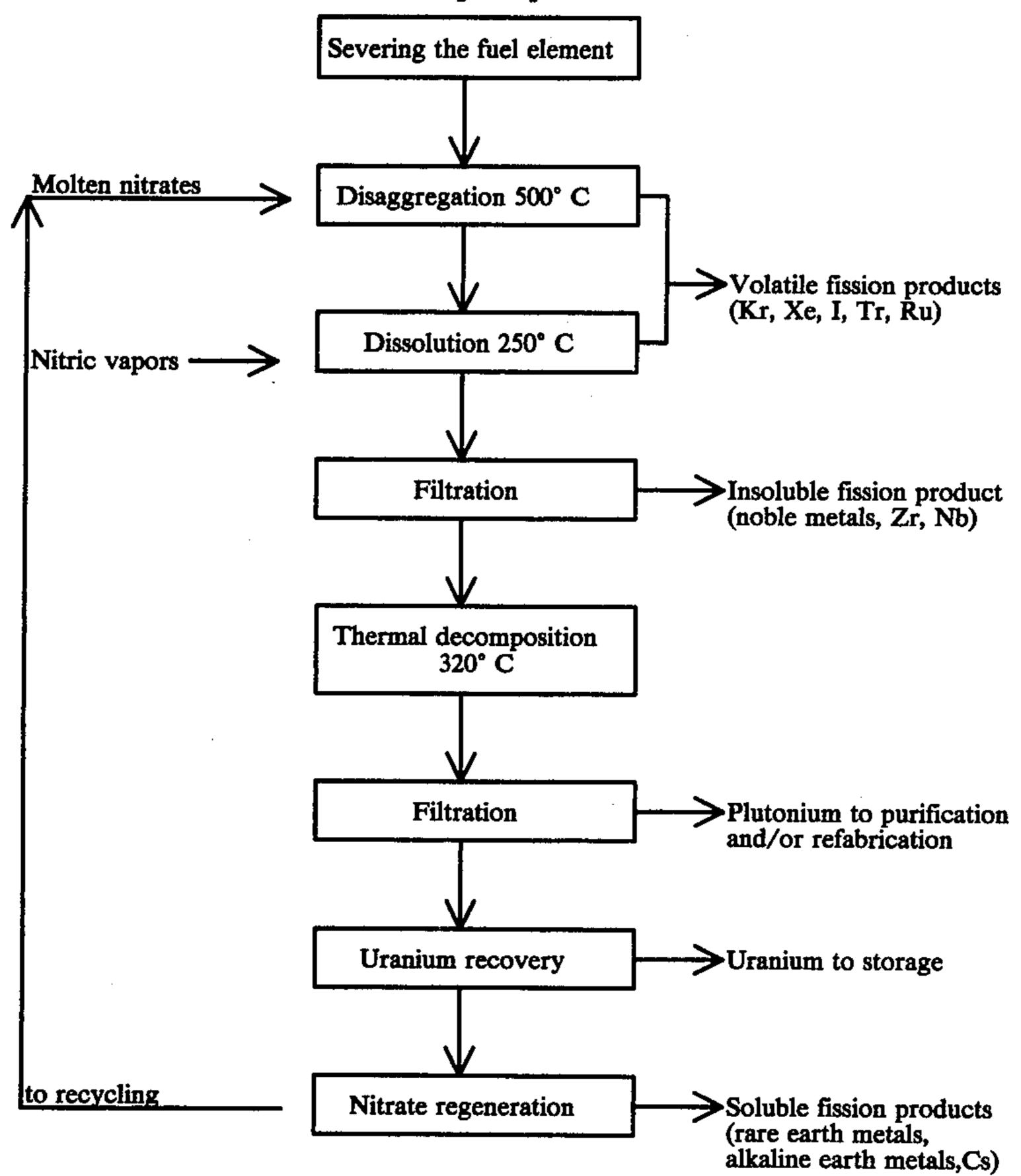
Block Diagram of the pyrochemical plutonium separation process.
