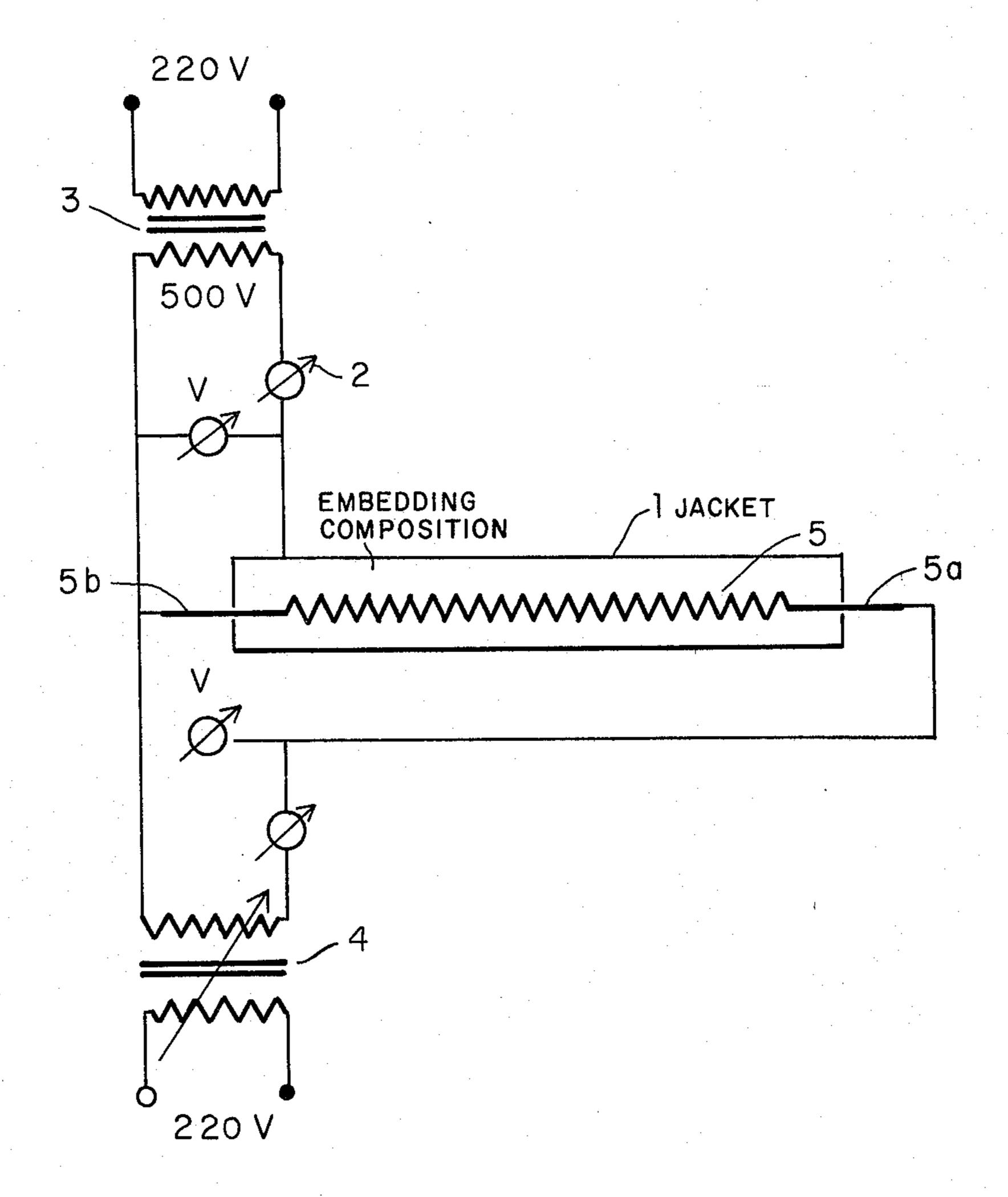
ELECTRICAL HEATING ASSEMBLY HAVING A THERMALLY CONDUCTIVE REFRACTORY ELECTRICAL INSULATING EMBEDDING COMPOSITION BETWEEN AN ELECTRICALLY CONDUCTIVE MEMBER AND A JACKET
