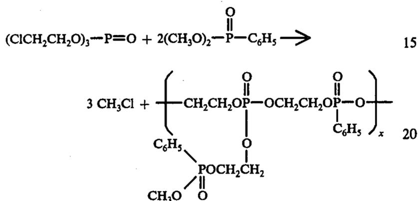
Reaction (K): tris( $\beta$ -chloroethyl)phosphate and dimethyl methyl phosphonate, 2 moles of phosphonate per mole of phosphate, with additionally 0.01 to 0.1 moles of dimethyl n-octadecyl phosphonate
