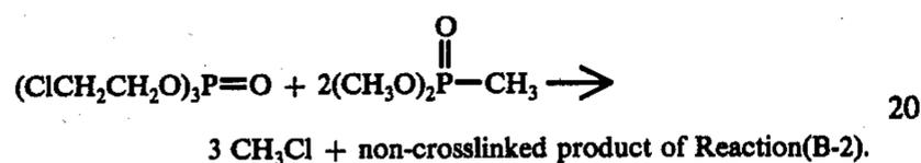
Reaction (D): tris( $\beta$ -chloroethyl) phosphate and dimethyl methyl phosphonate, 3 moles of phosphonate per mole of phosphate
