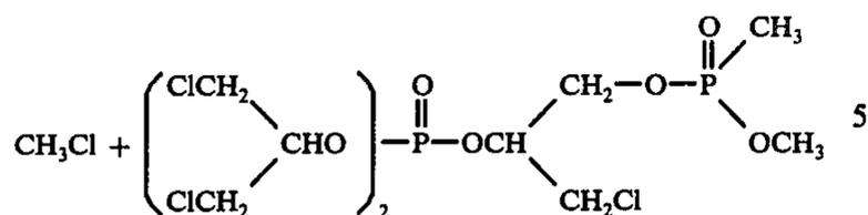
Reaction (J): tris( $\beta$ -chloroethyl) phosphate and dimethyl phenylphosphonate, 2 moles of phosphonate per moles of phosphate
