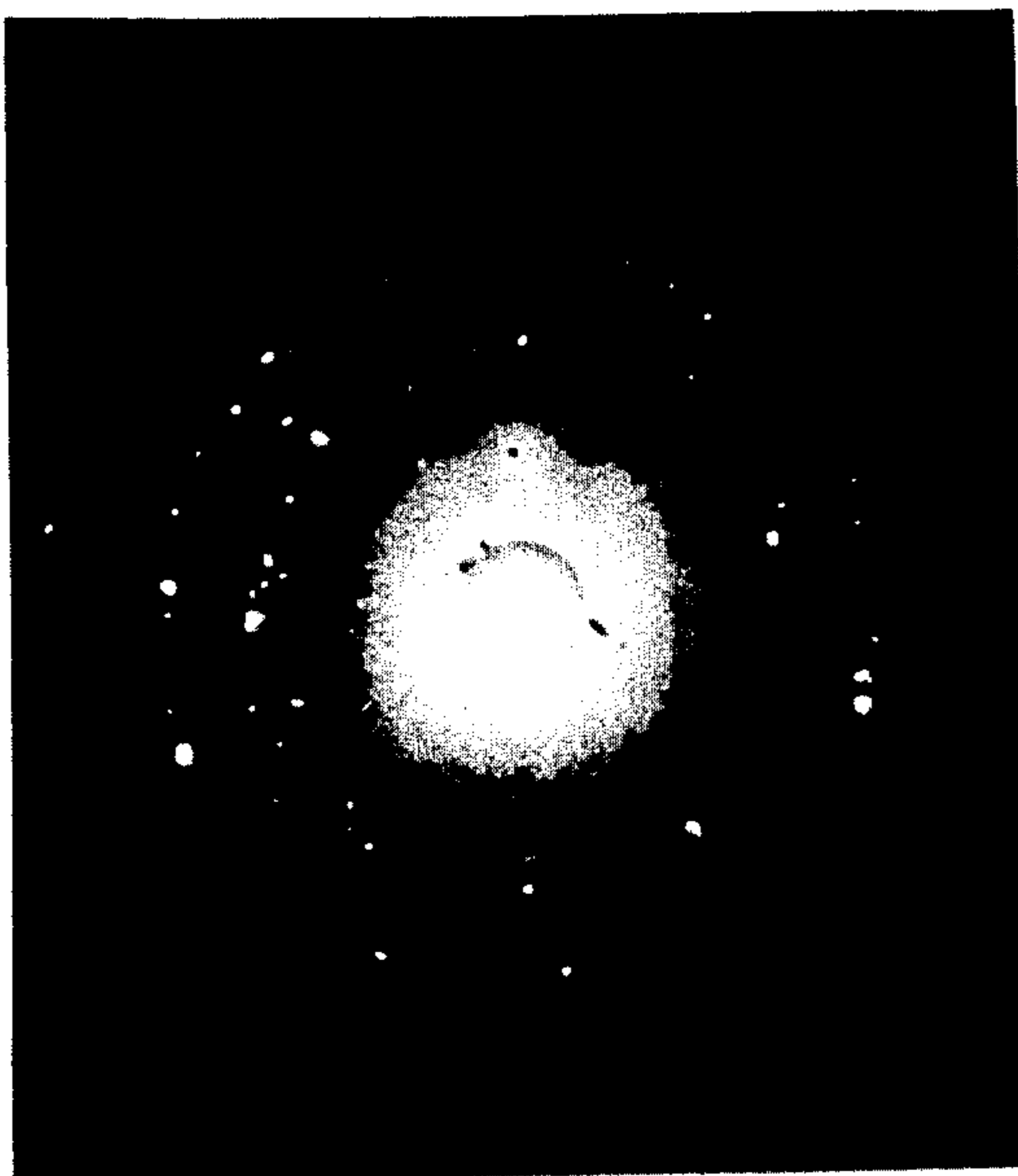
FIG. 14C AFTER ANNEALING FOR 1 HOUR AT 250°C
