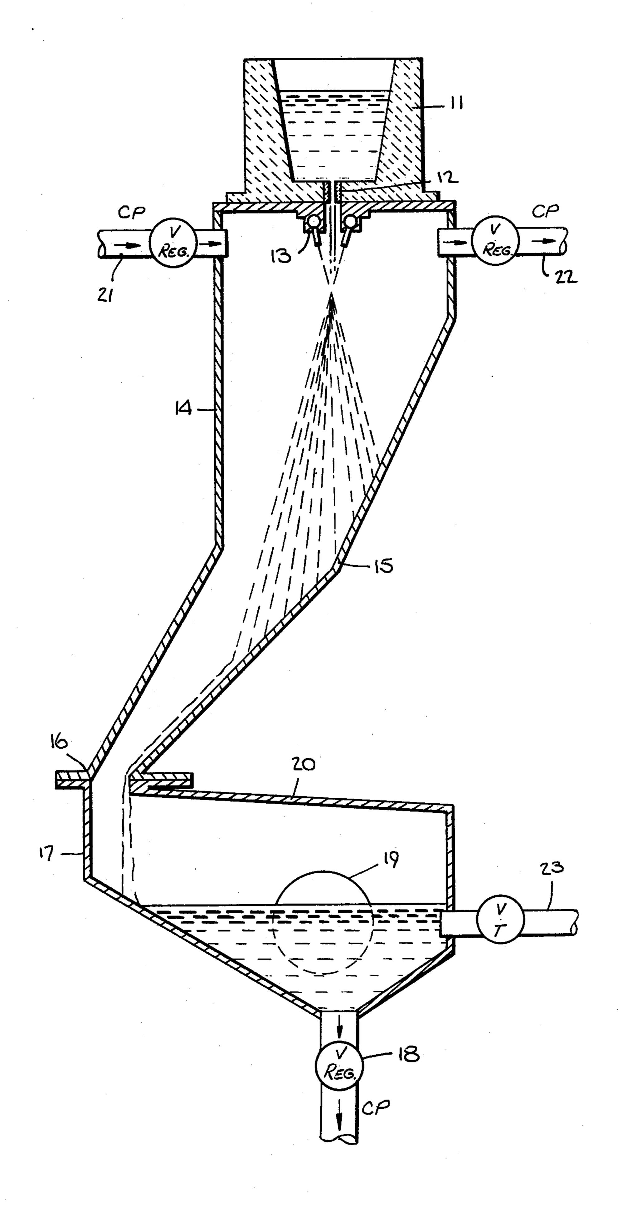
WATER ATOMIZER FOR LOW OXYGEN METAL POWDERS
