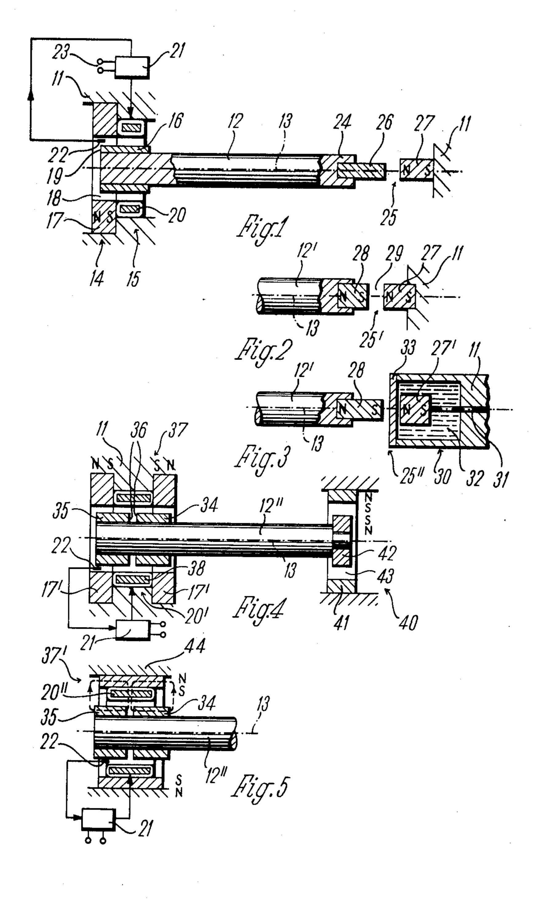
The invention relates to a magnetic bearing system for journalling a rotor on a stator without contact be- 5 tween the rotor and the stator, and more particularly to a magnetic bearing system having a passive axial bearing element which cooperates with a ferromagnetic
