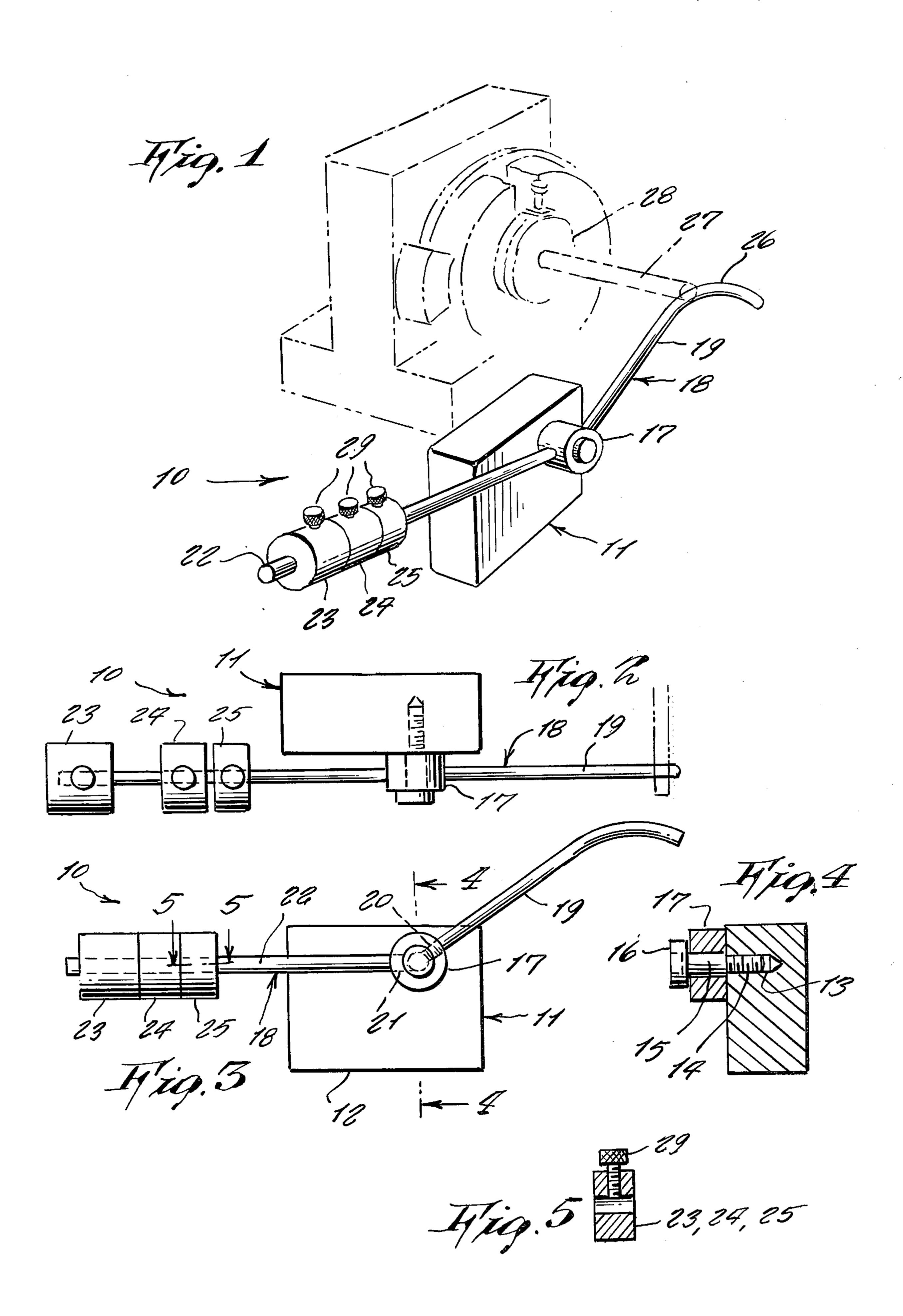
A cylindrically collar 17 is supported freely rotatable on the shoulder 15 of the screw.
