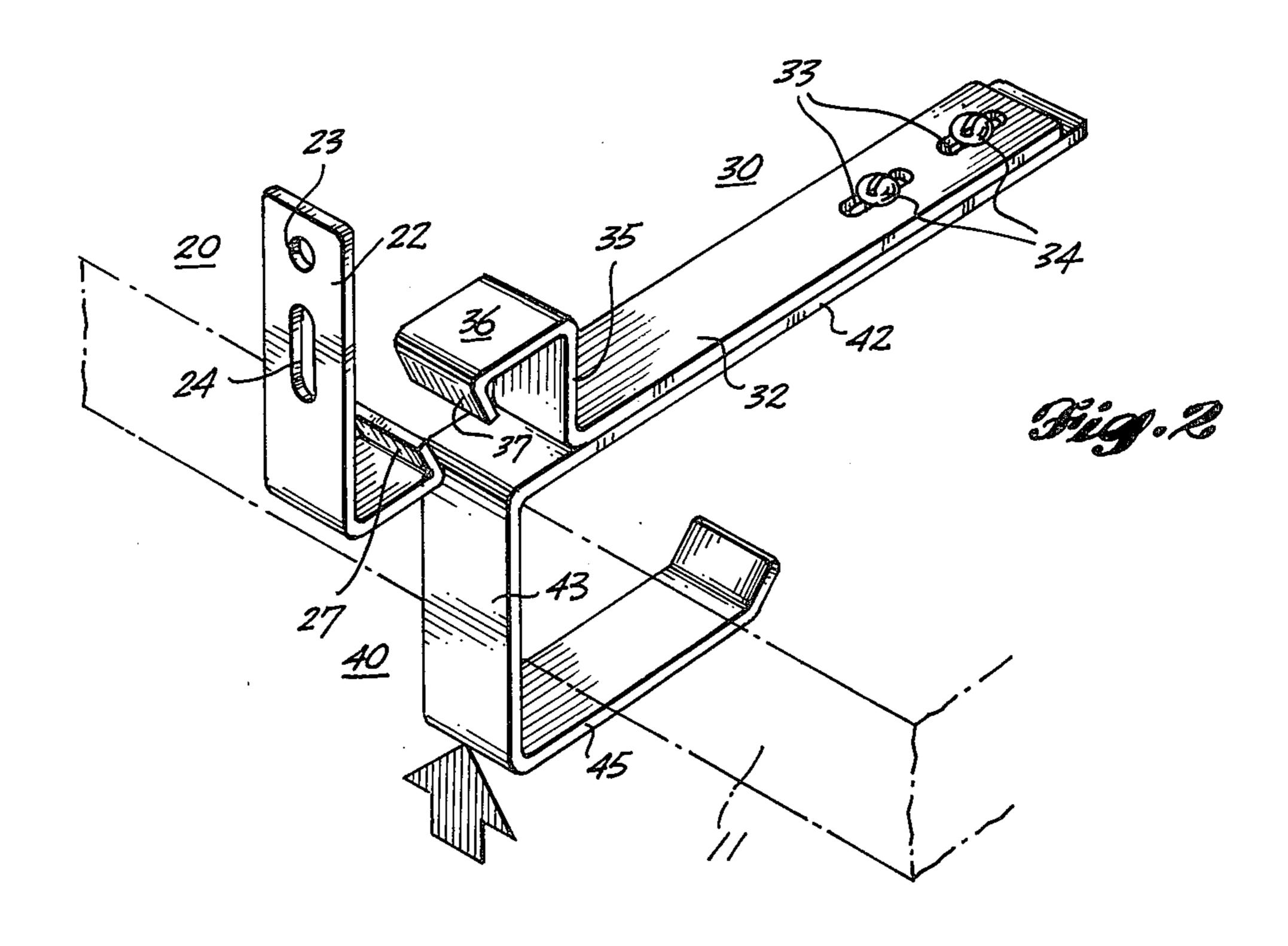
is associated with arm 26 at an acute angle to provide a wedging or lifting action as the door is being closed.
