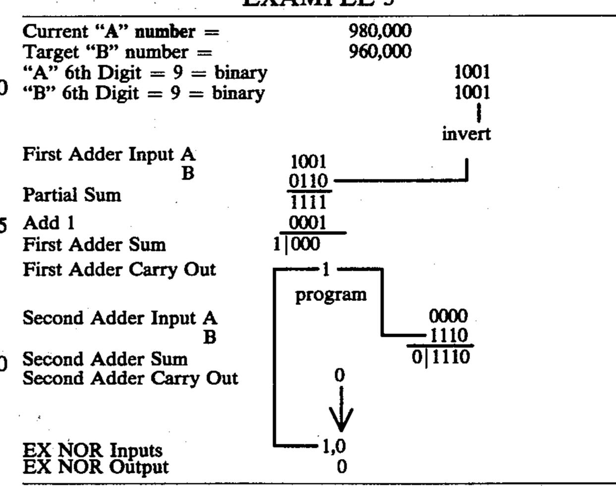
No reversal in scanning direction is required. The scan direction control will provide the down scan control signal at output 107 responsive to the second signal at output 105 of comparator 15.
