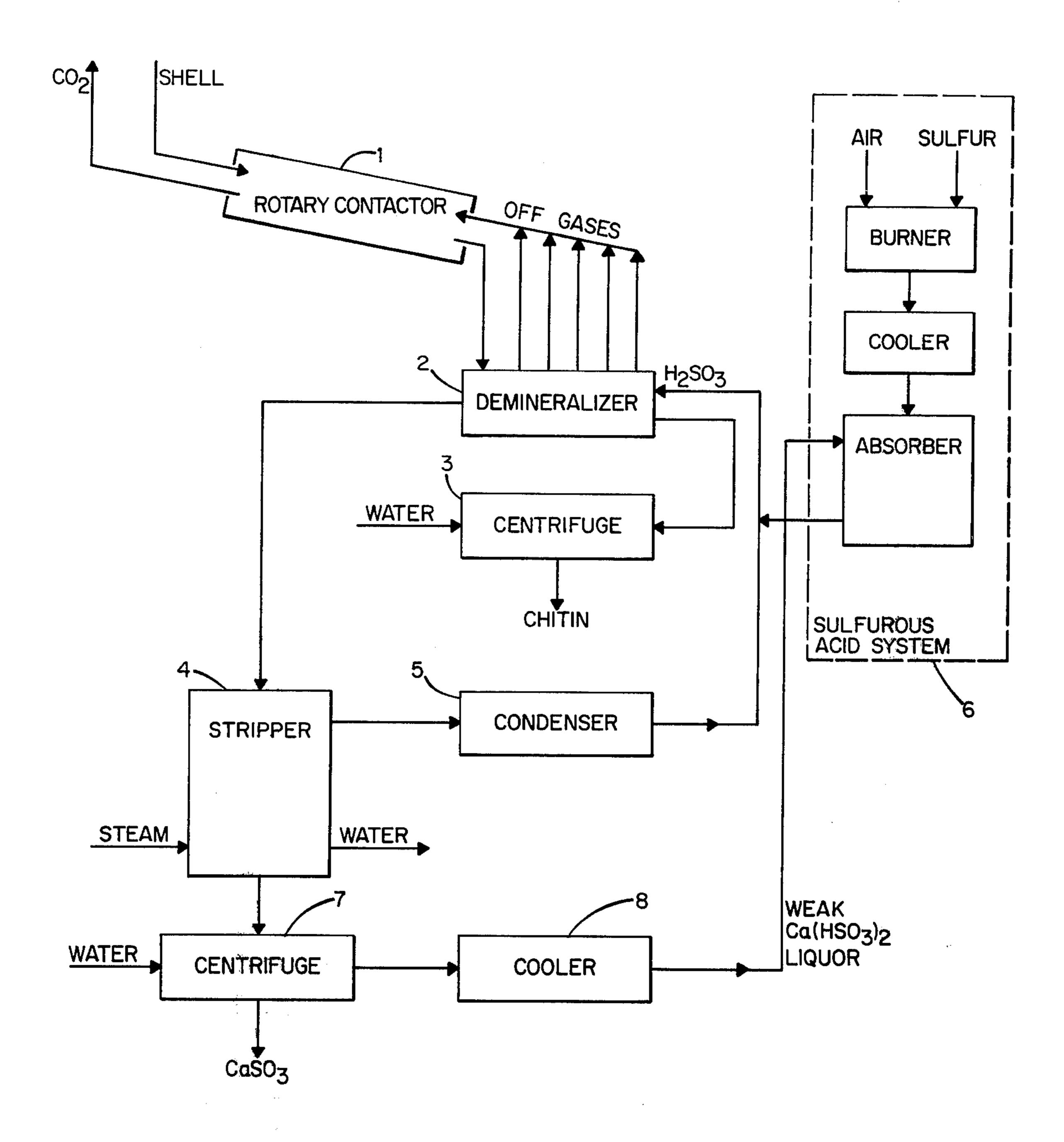
PROCESS FOR DEMINERALIZATION OF CRUSTACEA SHELLS
