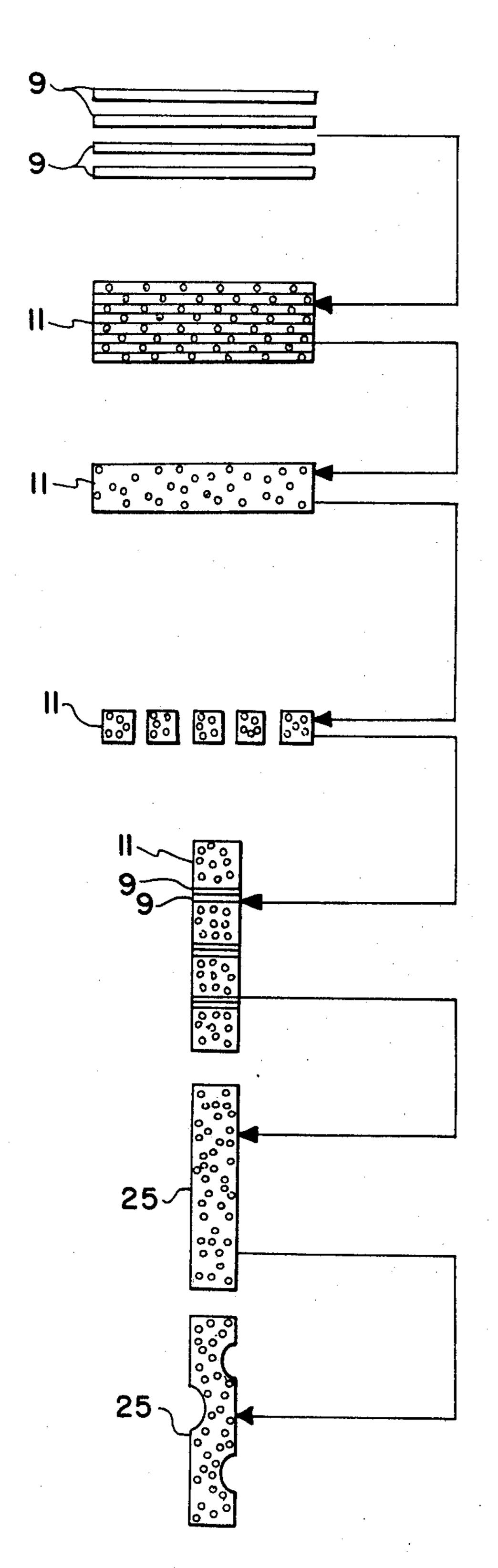
CUT A PLURALITY OF RESINIMPREGNATED FIBER TAPE INTO A PLURALITY OF DESIRED LENGTHS
