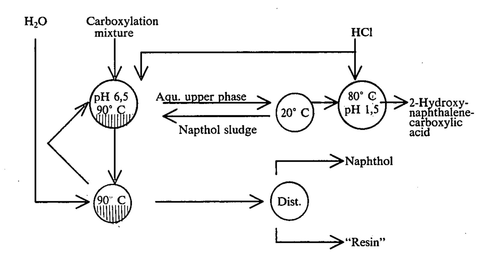
The organic phase is separated, likewise in known manner, by distillation under reduced pressure in pure re-usable 2-hydroxynaphthalene (distillate) and waste 50 products (sump).
