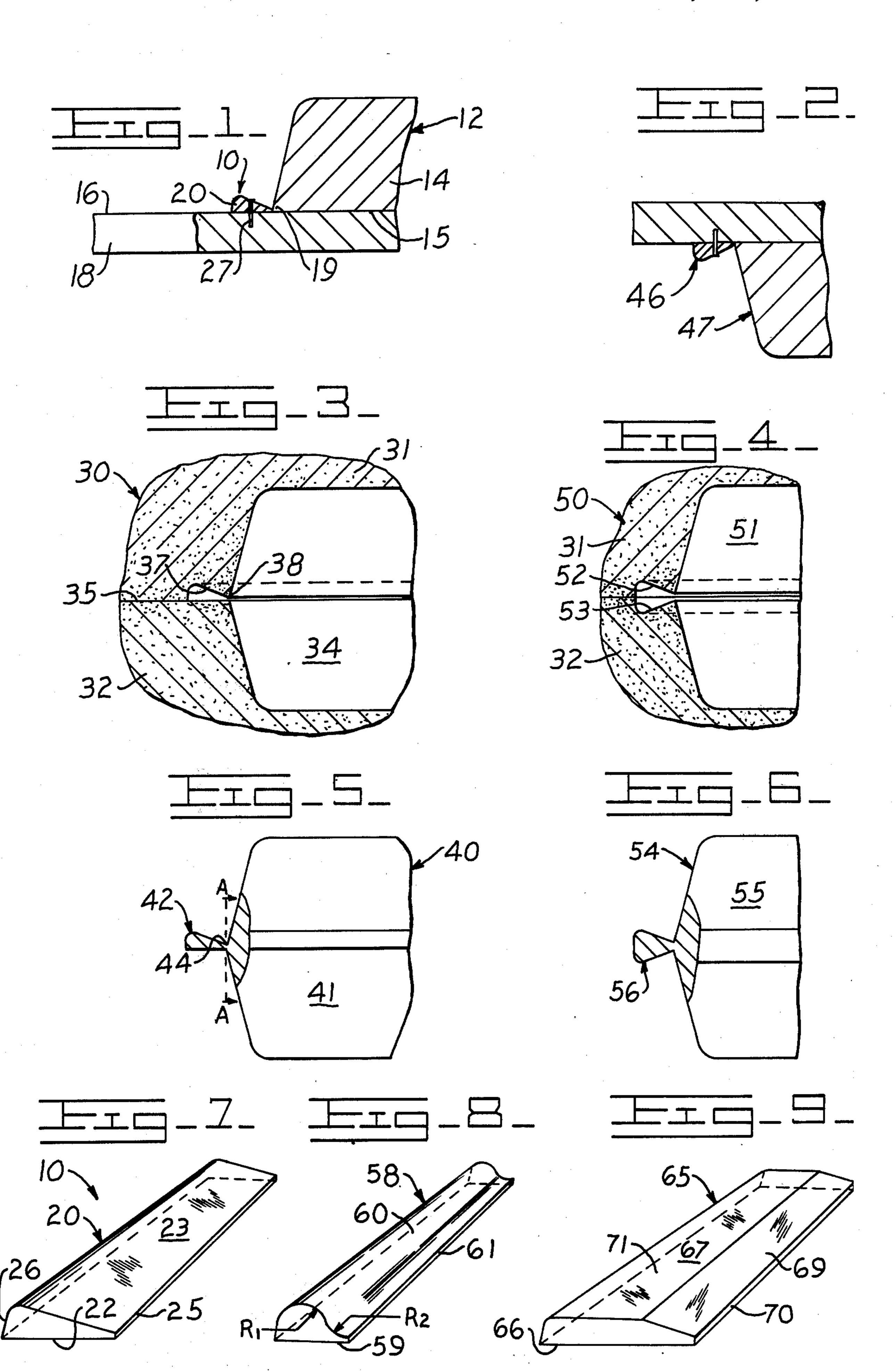
so as to produce controlled shape flash which has a built-in fracture line contiguous to the casting so that the flash is cleanly and easily removed from the casting.
