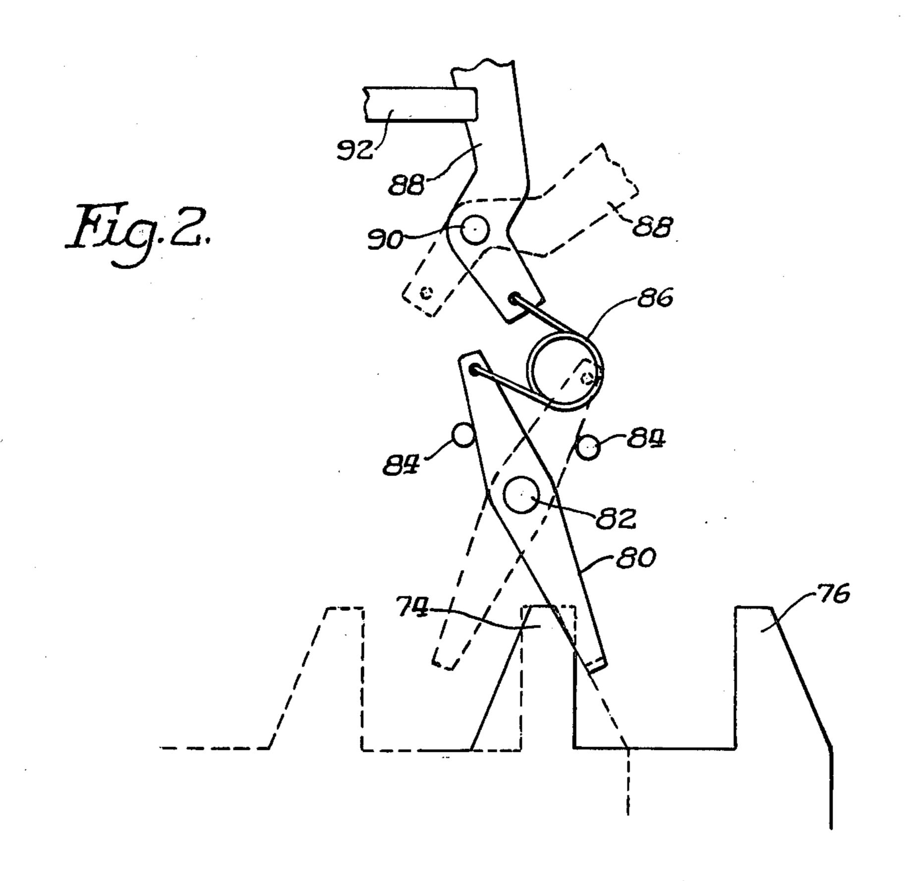
STARTING AND STOPPING DEVICE FOR SOUND MOTION PICTURE CAMERA
