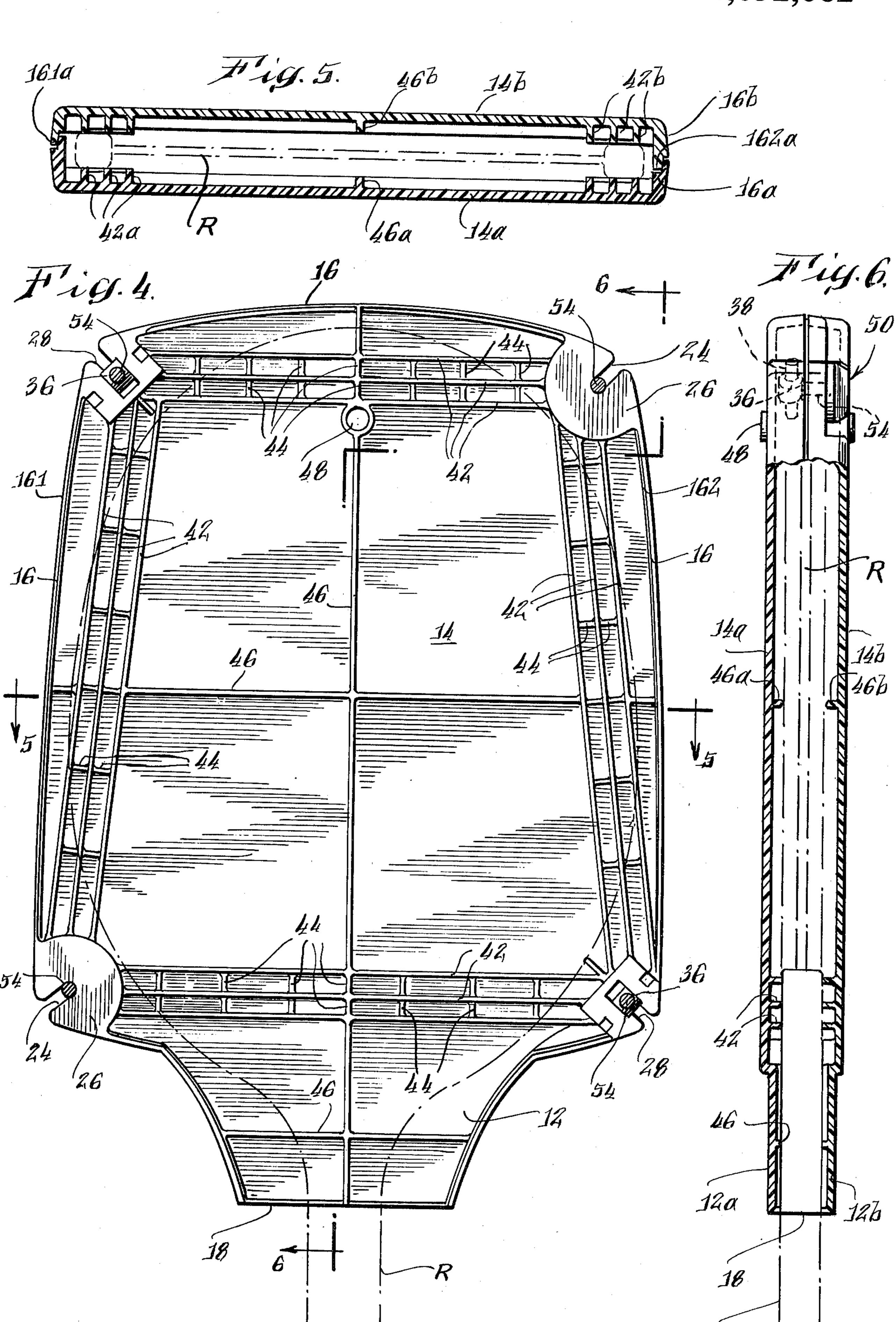
FIG. 6 is a cross section taken substantially along the line 6—6 of FIG. 4, also showing both half members.
