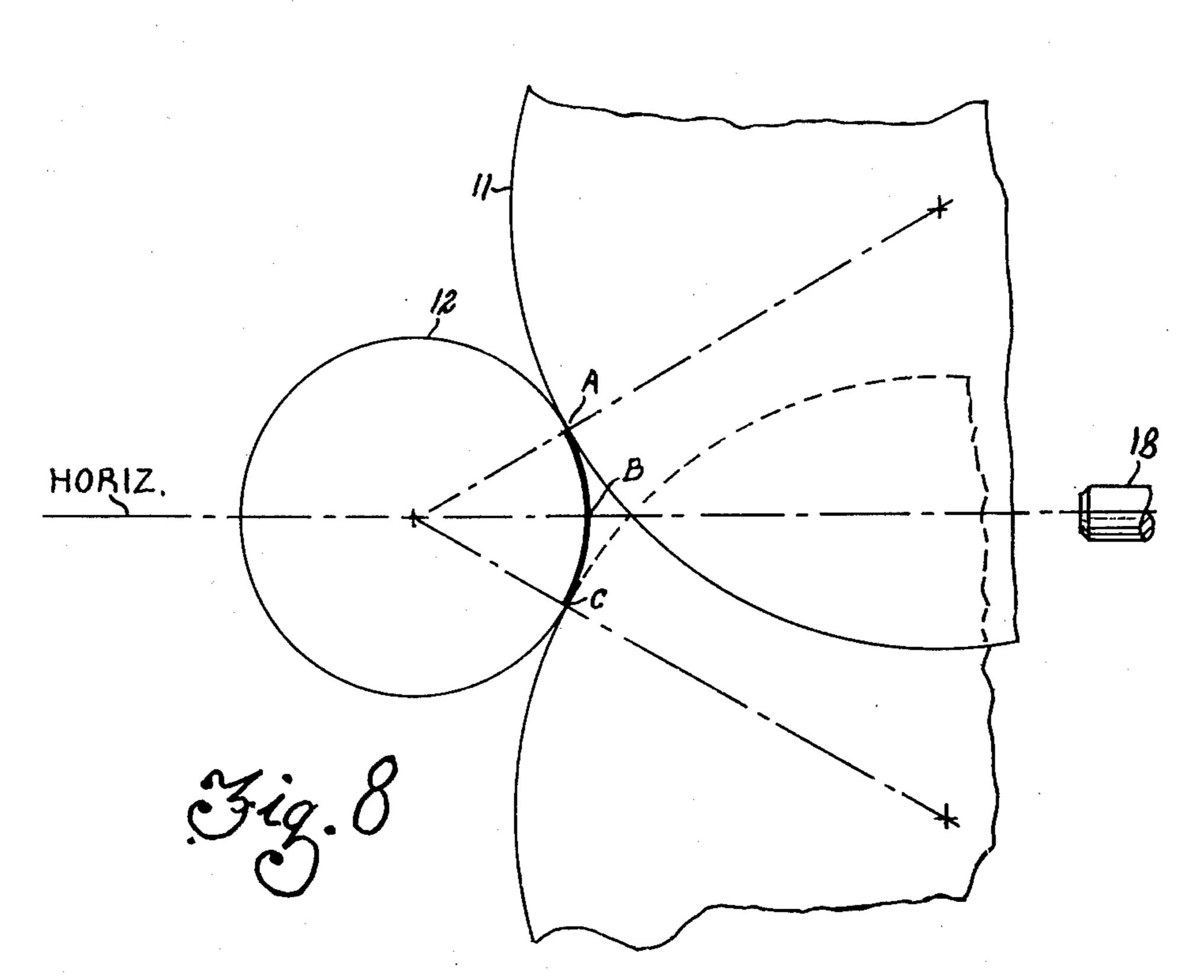
REGULATING WHEEL PIVOT ADJUSTING **DEVICE**
