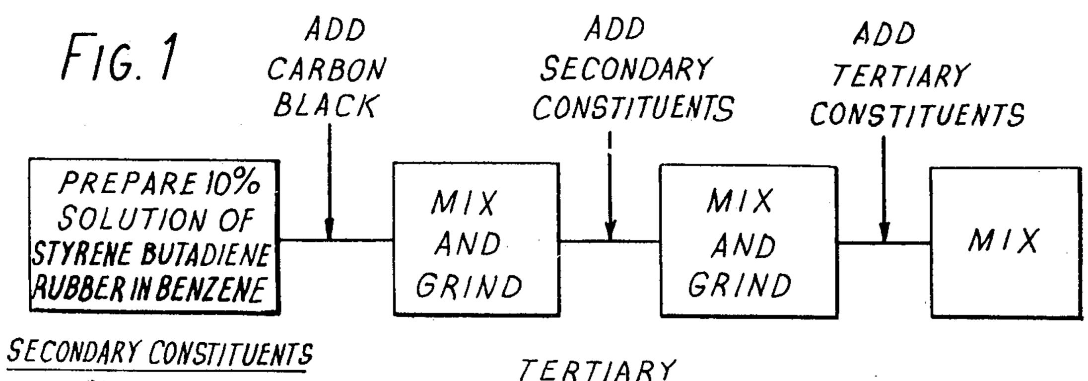
SULFUR BENZOTHIAZYLDISULFIDE ZINC OXIDE, STEARIC ACID, ANTIOXIDANT, ACCELERATOR TERTIARY CONSTITUENTS
