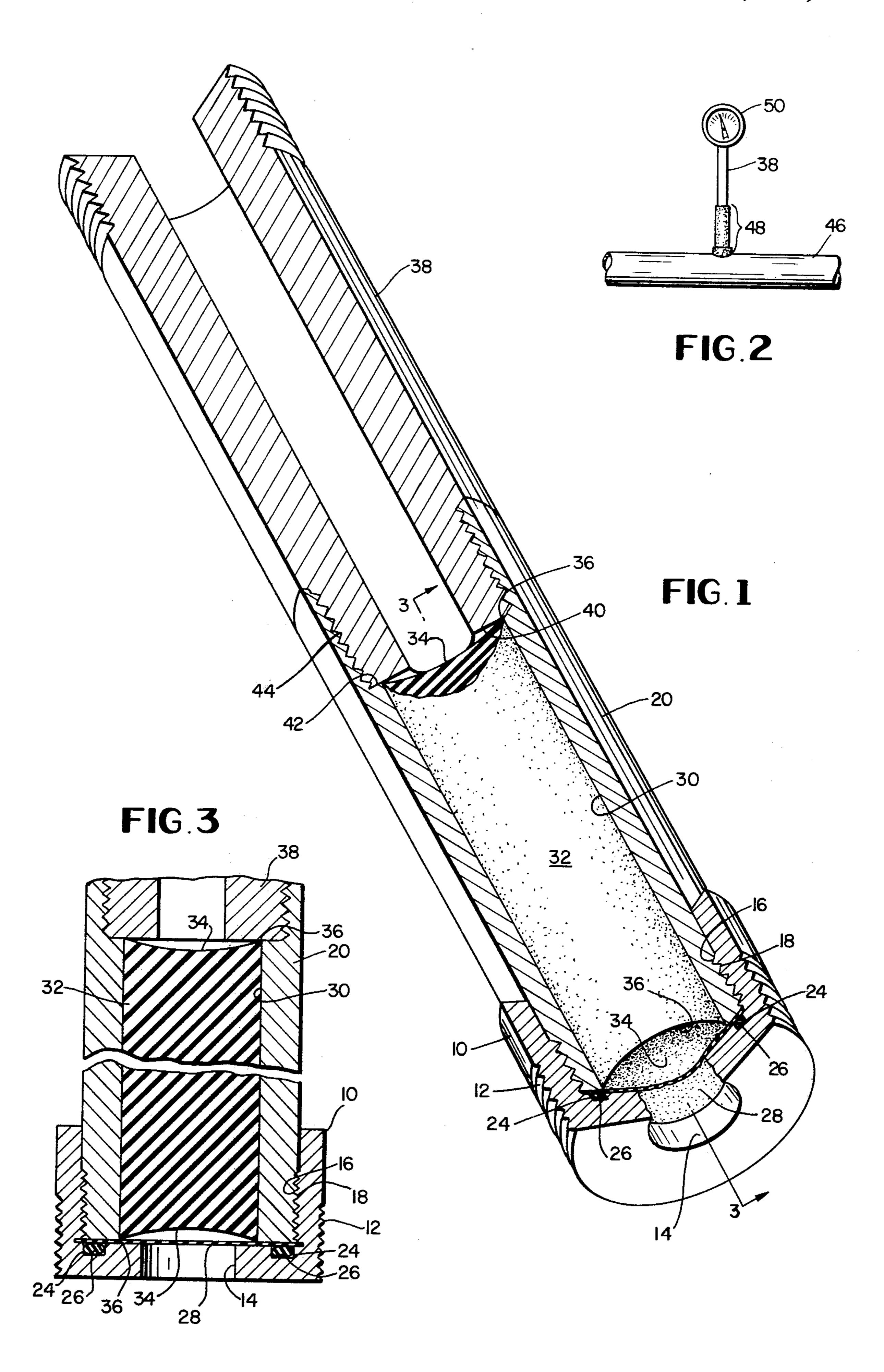
An O ring 26 made of neoprene or other suitable material is fitted in the groove 24 and a round flexible diaphragm 28 made from rubber, neoprene or other
