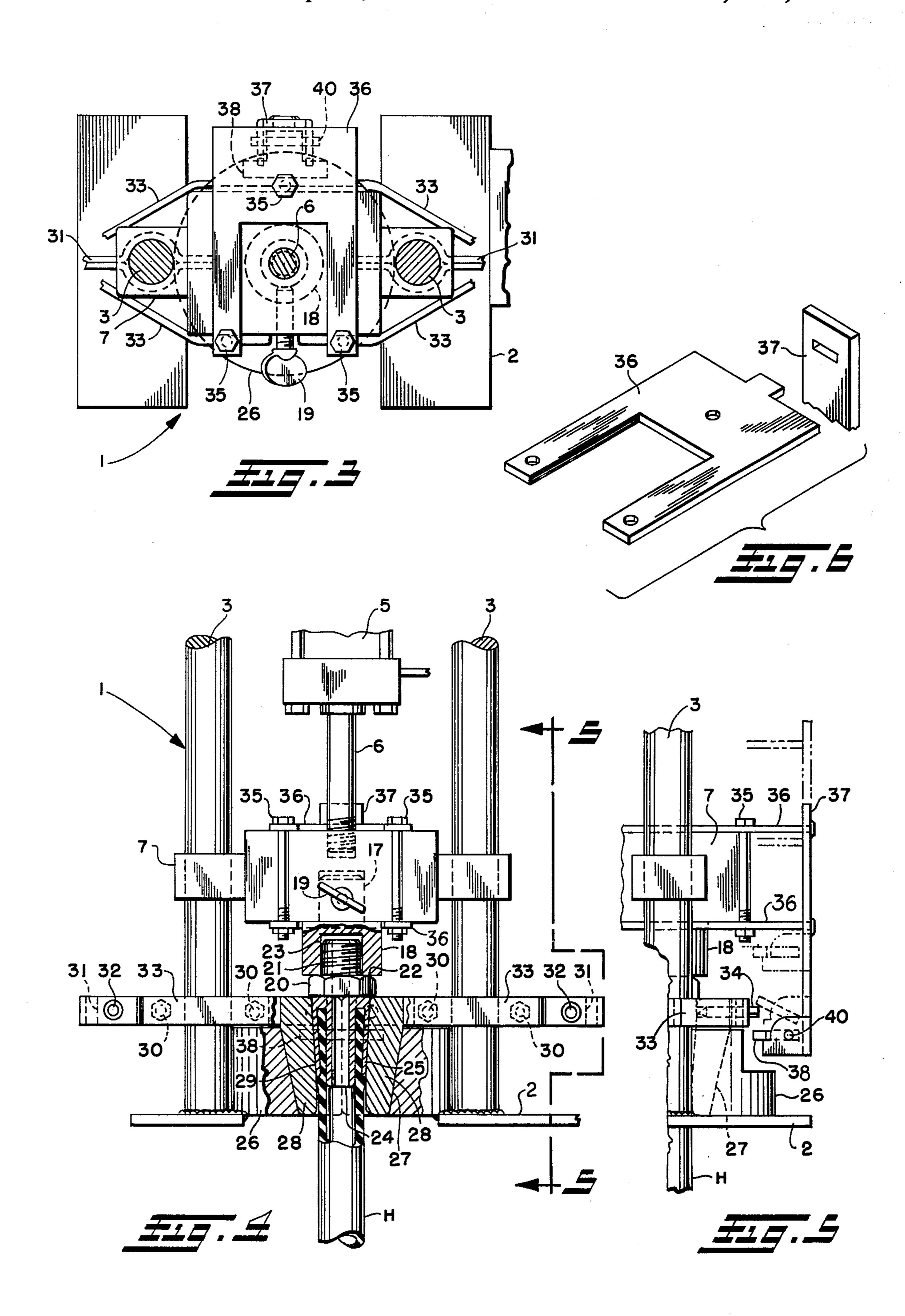
lifting and lateral separation of the die members during the retraction of the pusher.
