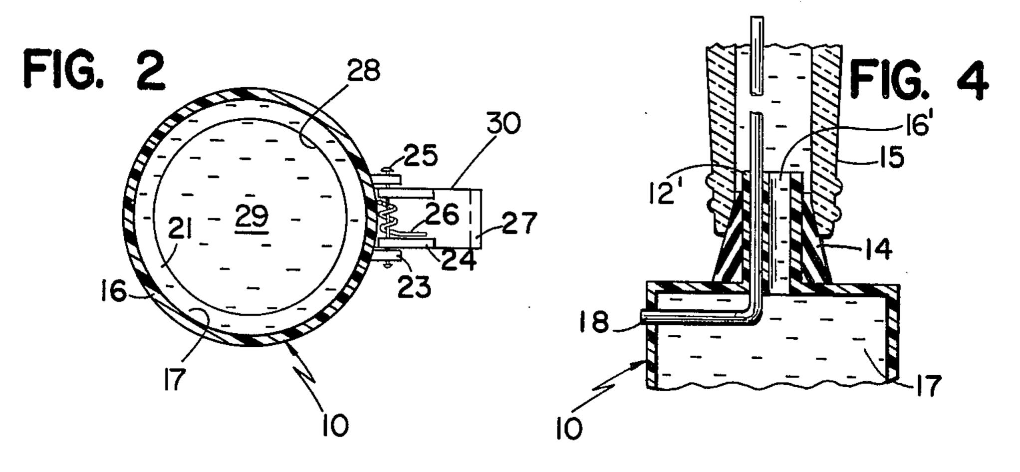
Spring 26 biases cover 29 to a closed position over aperture 28. A lever 30, integral with cover 29, extends beyond the hinge connection of cover 29 to housing 10 and preferably includes an upstanding lip 27 thereon.
