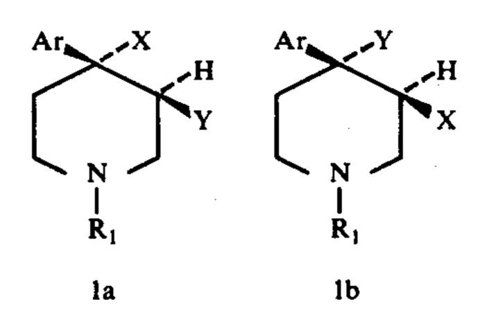
wherein R<sub>1</sub> and Ar are as defined broadly above and X is R<sub>2</sub> or R<sub>3</sub> when a free or protected hydroxyl group, and Y is R<sub>2</sub> or R<sub>3</sub> when cyano, or a free amino or a derivative thereof.
