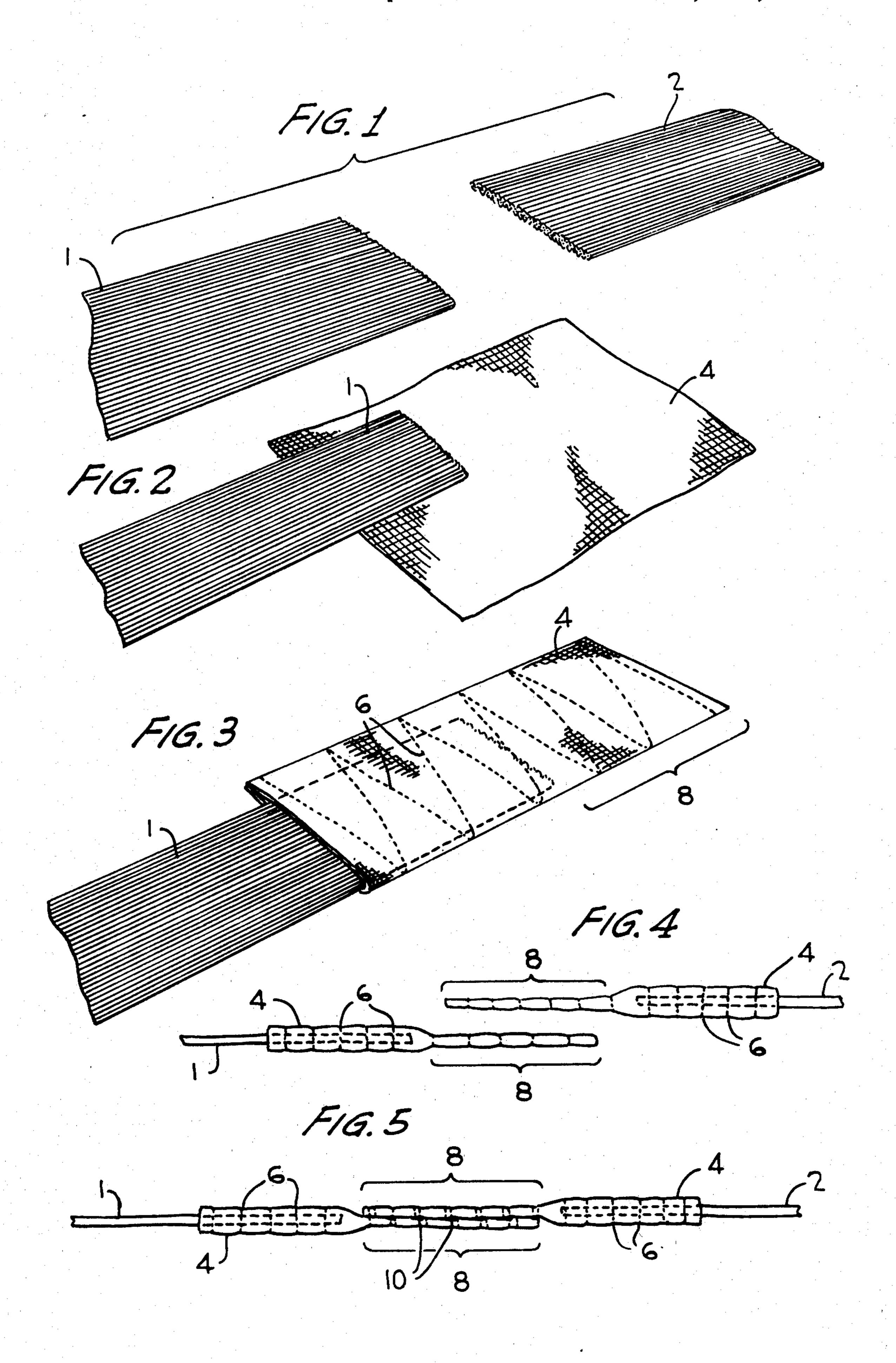
SPLICE FOR USE DURING THE THERMAL STABILIZATION OF A FLAT MULTIFILAMENT BAND OF AN ACRYLIC FIBROUS MATERIAL COMPRISING AT LEAST TWO SEGMENTS
