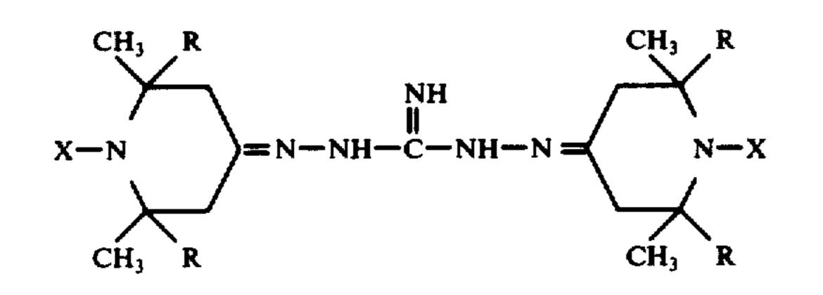
wherein X is —H, —OH, —0., alkyl of 1 to 8 carbon atoms, or carboxylic acyl of 2 to 10 carbon atoms, and R is alkyl of 1 to 8 carbon atoms.
