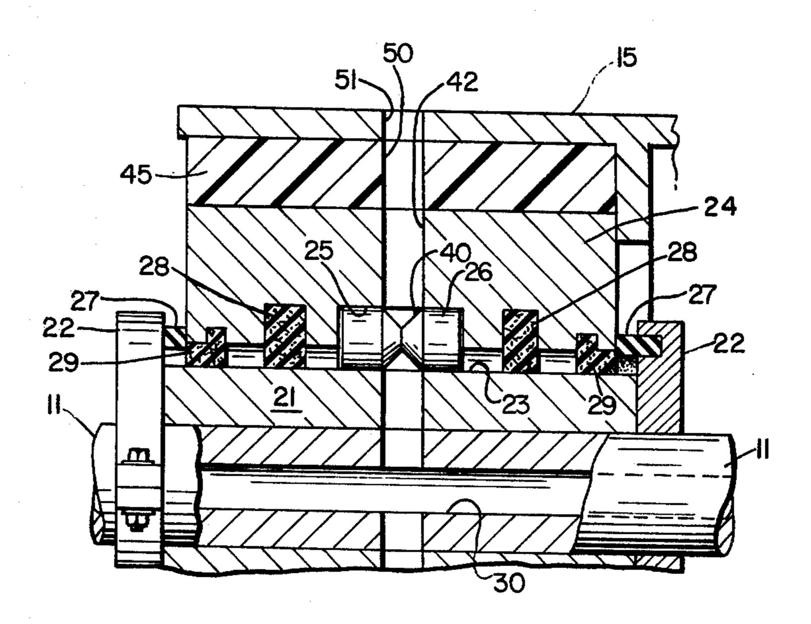
WATER LUBRICATED BEARING ASSEMBLY FOR
