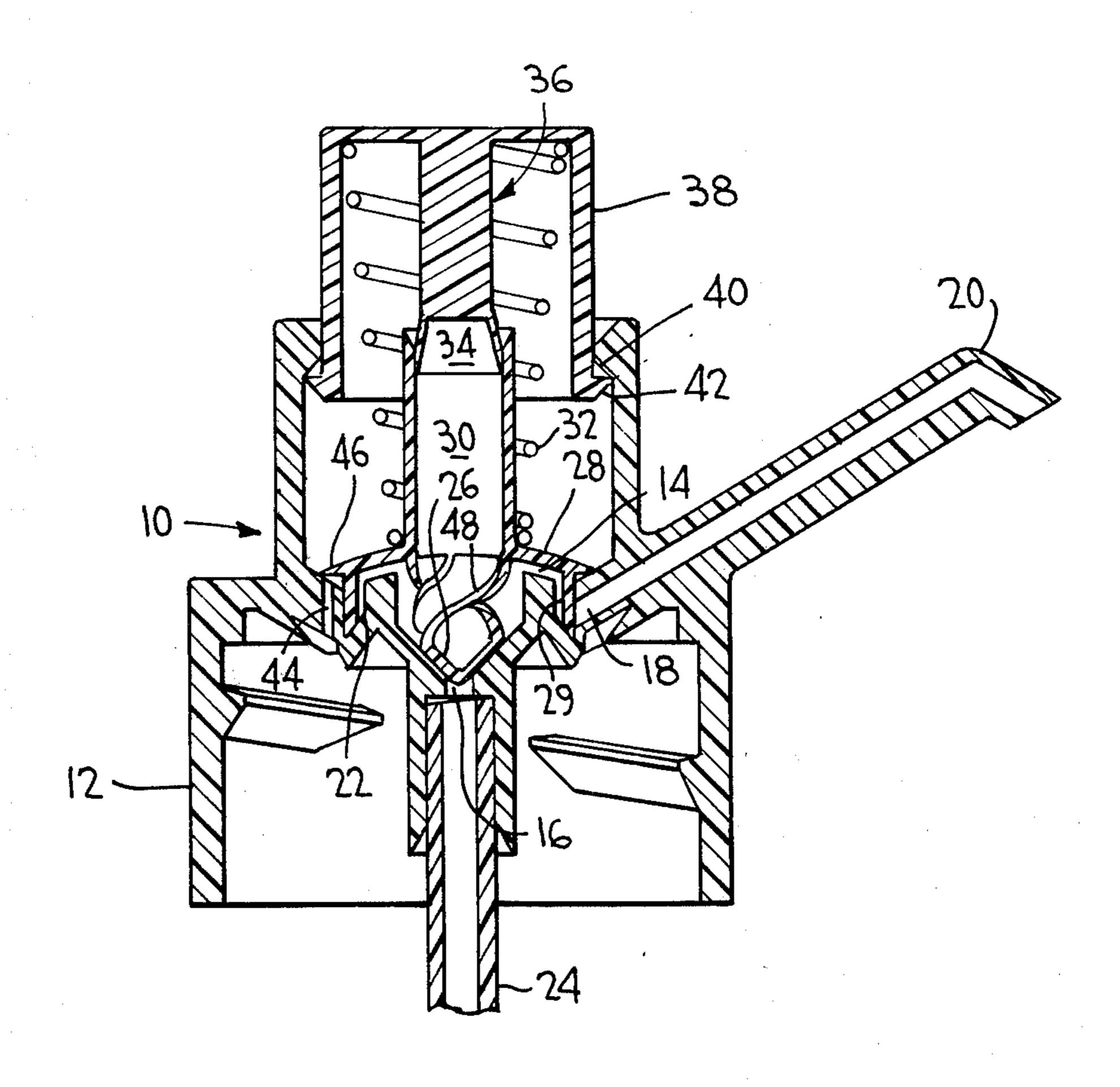
This invention relates to improvements in a dispensing pump of the class of which the pump cylinder communicates with and delivers liquid under pressure into a pressure accumulation chamber from which the discharge of pressurized product to the atmosphere is under the control of an outlet valve which permits discharge only when a predetermined minimum dis- 10 charge pressure exists in the accumulation chamber.
