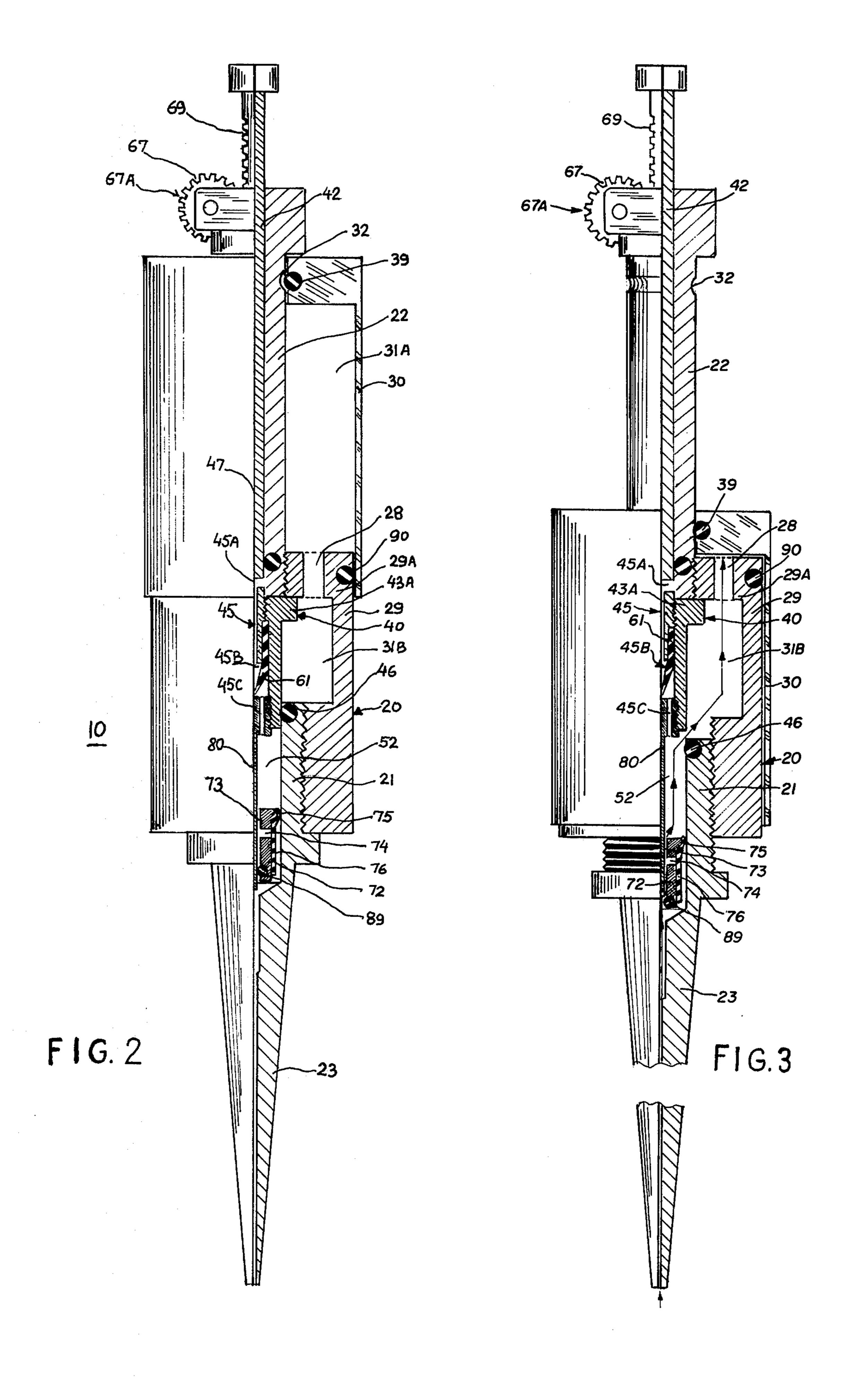
DEVICE FOR PIPETTING AND/OR DILUTING
