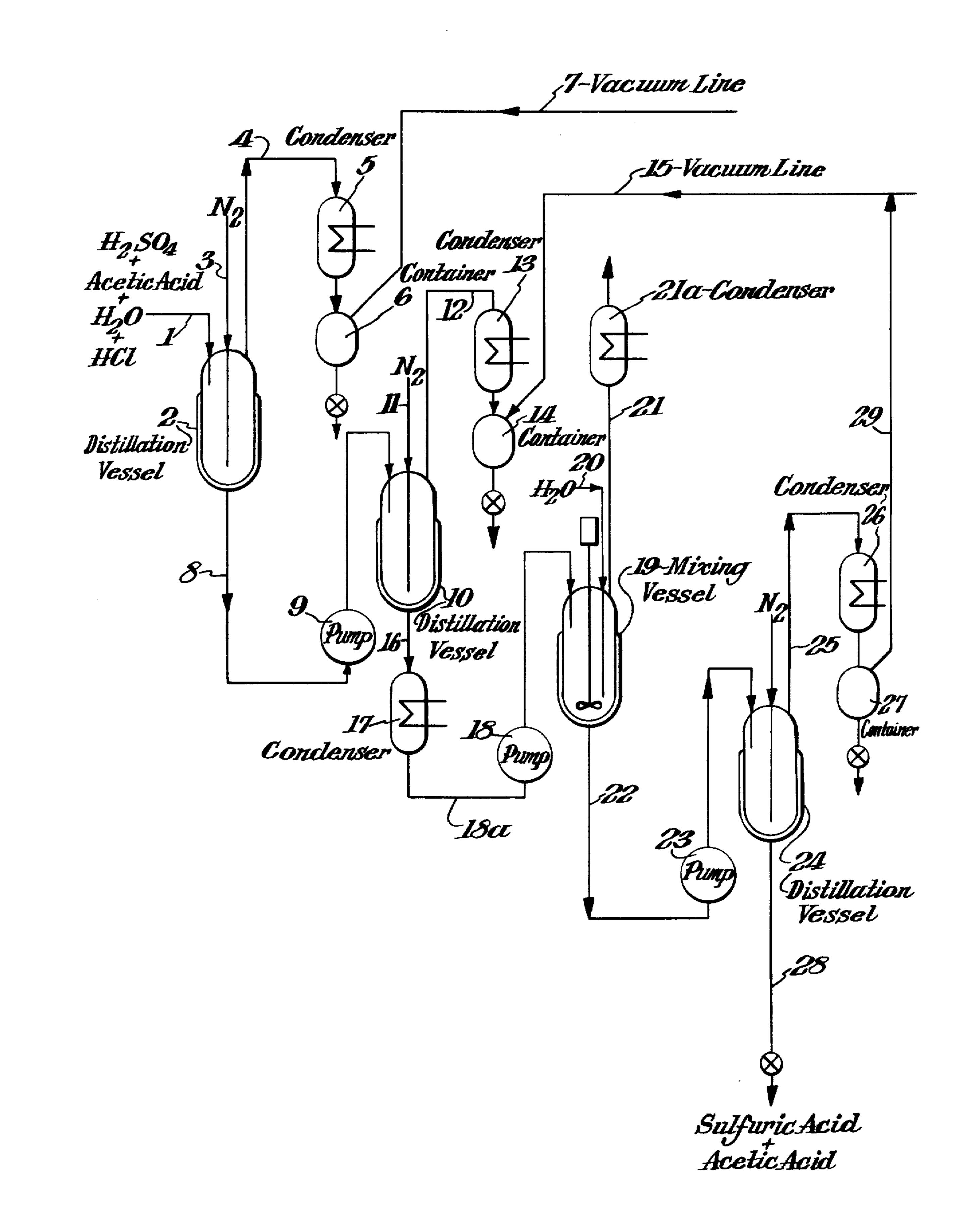
We have now unexpectedly found that it is possible for acetic acid to be separated from a mixture with sulfuric acid by distillative treatment under specific conditions which substantially avoid partial decomposi-
