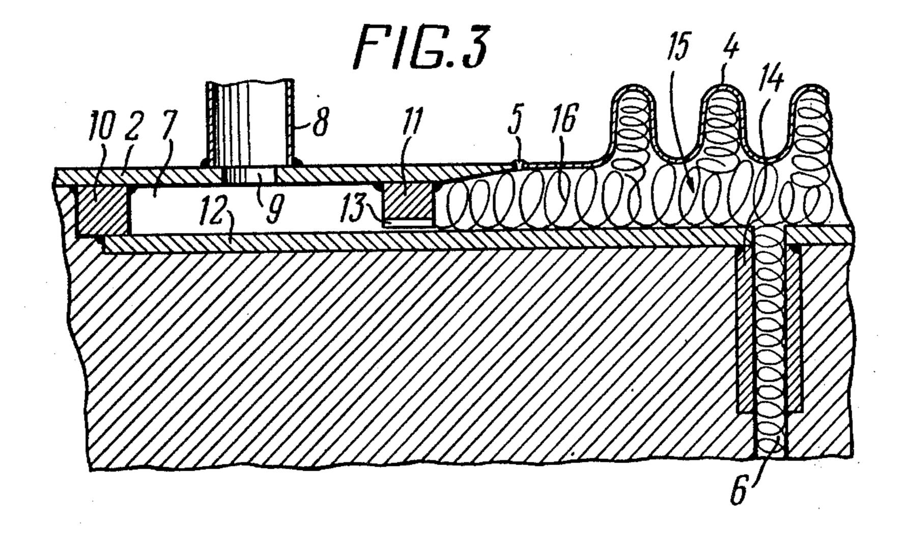
EXPANSION COMPENSATOR FOR PIPELINES
