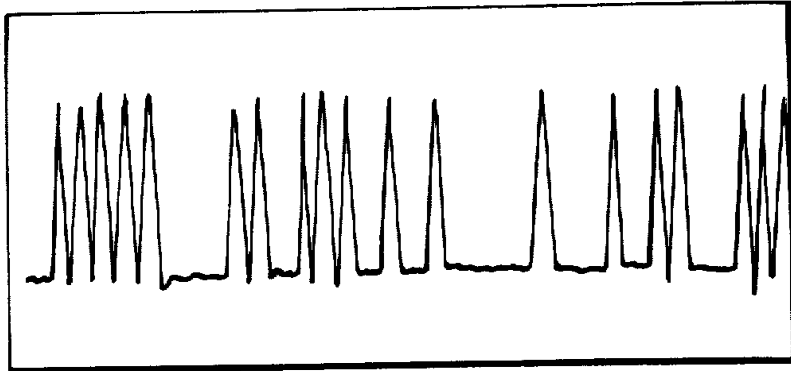
P 1 POLARIZATION WORST CASE DYNAMIC EXTINCTION RATIO ≥ 22.4:1
