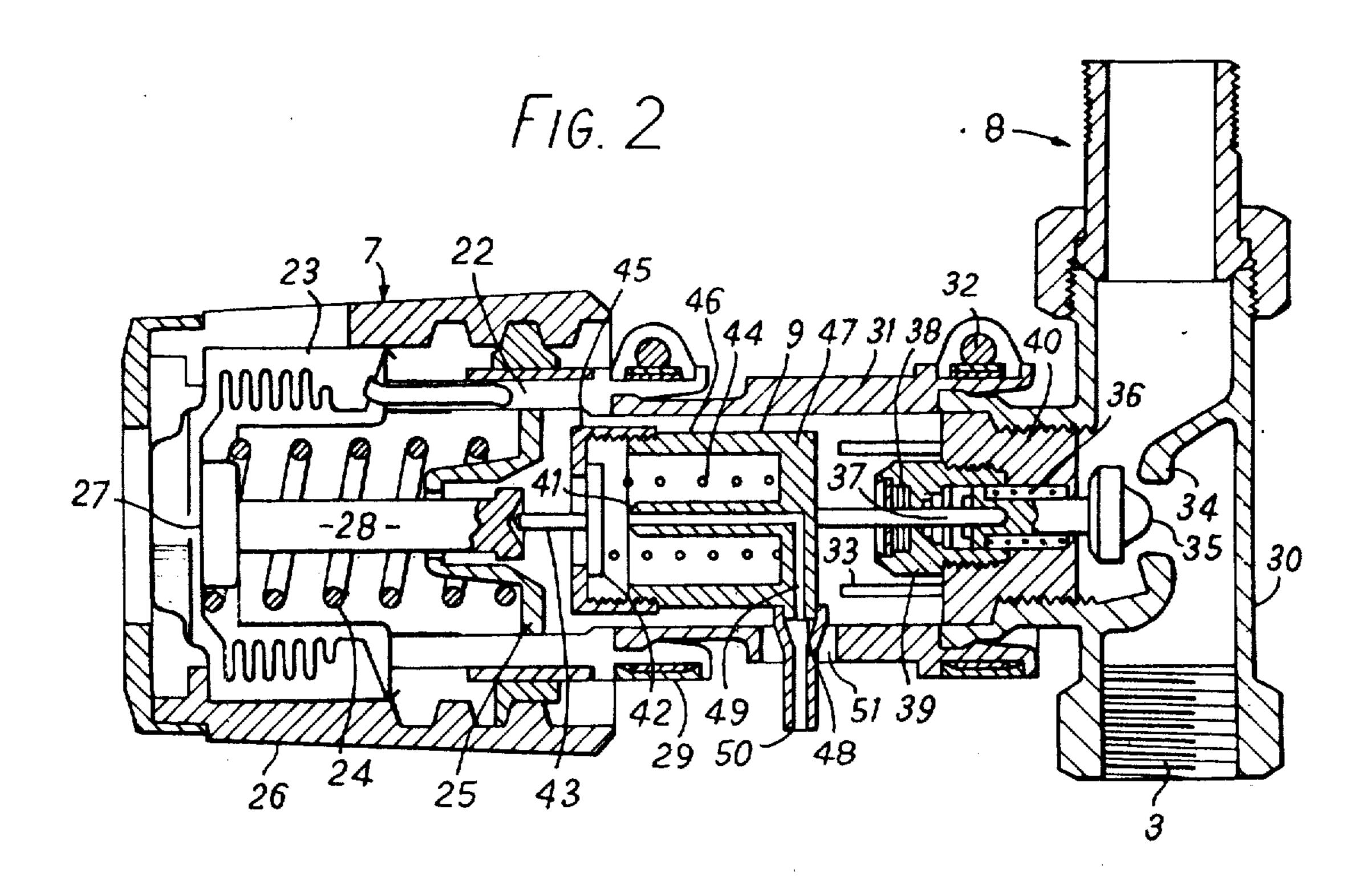
THERMOSTATIC REGULATING MEANS FOR AN AIR-CONDITIONING PLANT
