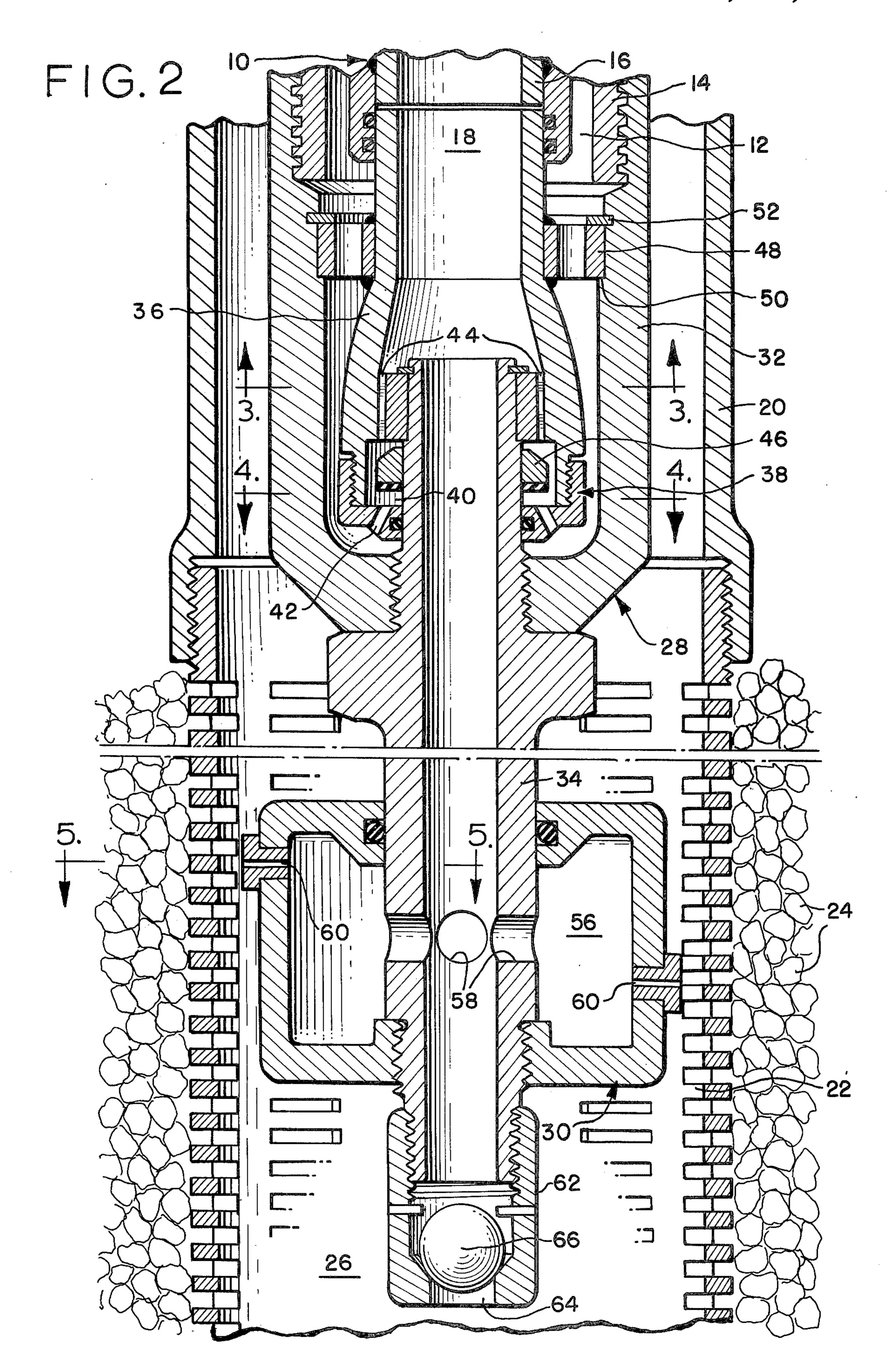
METHOD AND APPARATUS FOR CLEANING A SCREENED WELL
