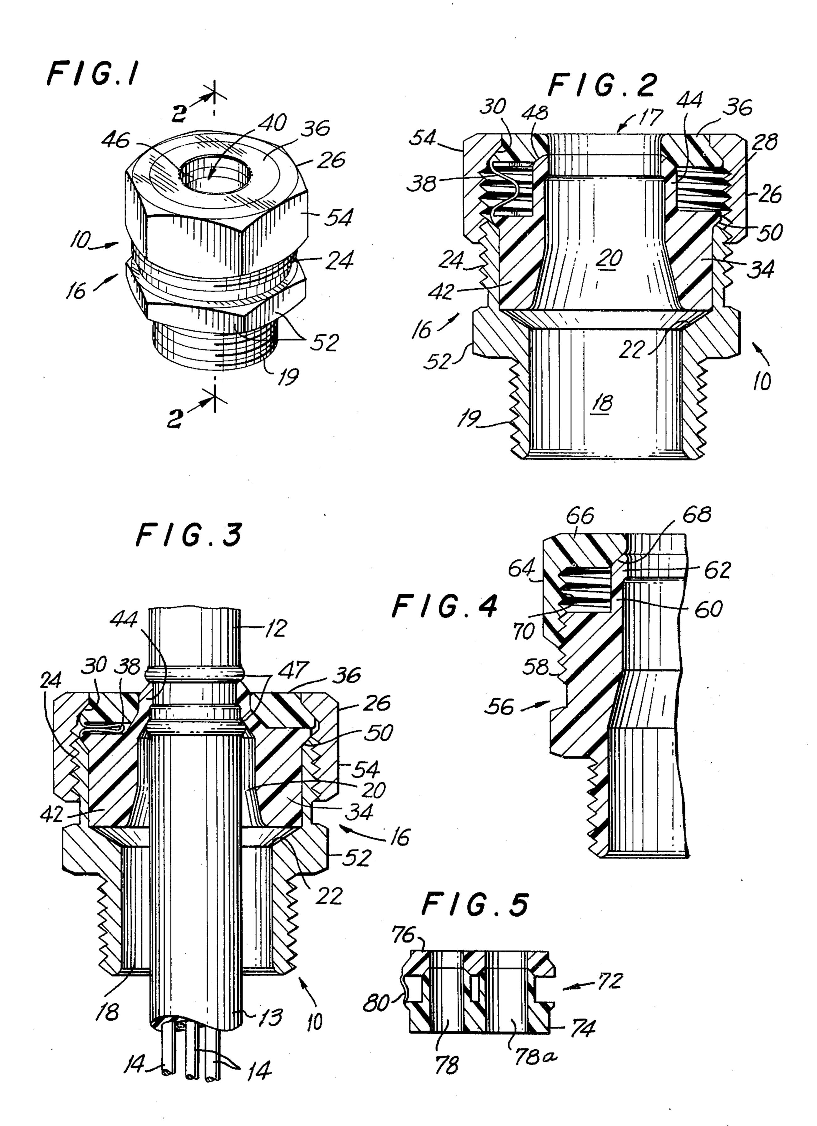
FITTING FOR CONDUIT AND ELECTRICAL CABLE
