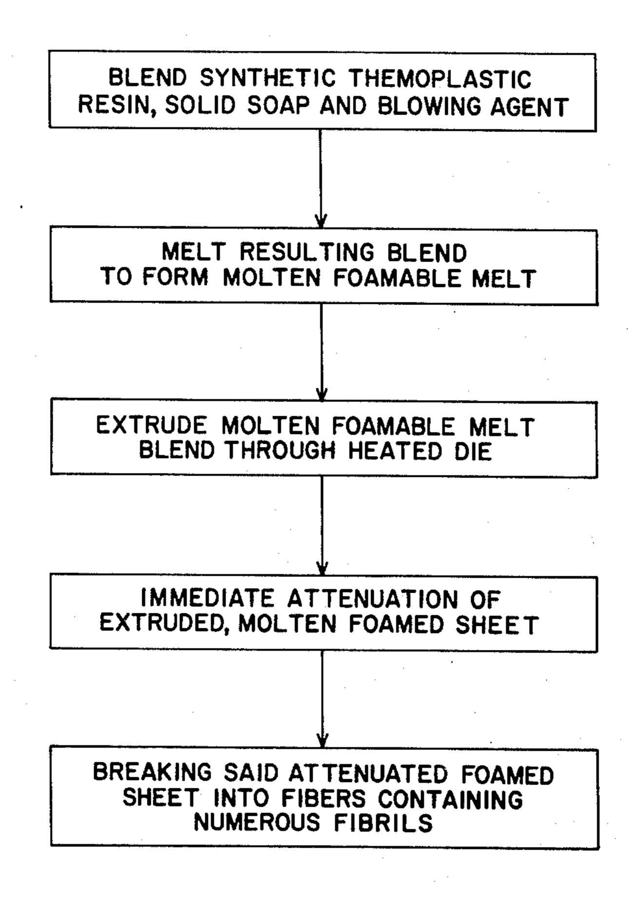
BLEND SYNTHETIC THEMOPLASTIC RESIN, SOLID SOAP AND BLOWING AGENT MELT RESULTING BLEND TO FORM MOLTEN FOAMABLE MELT EXTRUDE MOLTEN FOAMABLE MELT BLEND THROUGH HEATED DIE IMMEDIATE ATTENUATION OF EXTRUDED, MOLTEN FOAMED SHEET BREAKING SAID ATTENUATED FOAMED SHEET INTO FIBERS CONTAINING NUMEROUS FIBRILS
